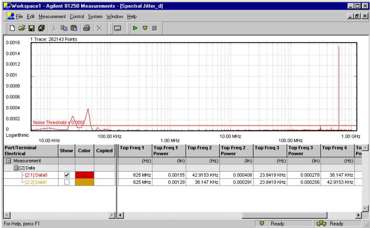
Thanks to the better resolution, you can see that the low frequency jitter component of the terminal “Data0” is actually composed of two frequencies.
