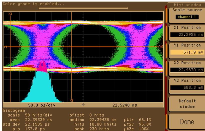
Deterministic jitter periodically adds and subtracts a delay to/from the received signal.
