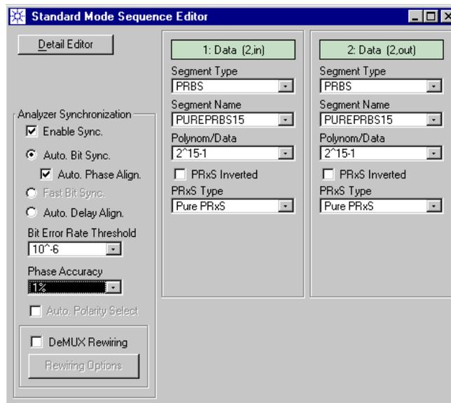
*Automatic Bit Synchronization with Automatic Phase Alignment* ensures that the analyzers will position their sampling point
