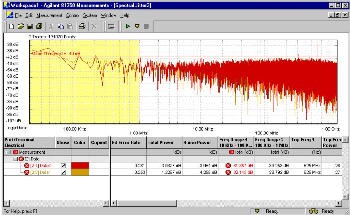
You can see how the frequency ranges are highlighted. Their settings and results are displayed in the numerical section. The total spectral power of Frequency Range 1 exceeds the maximum.
