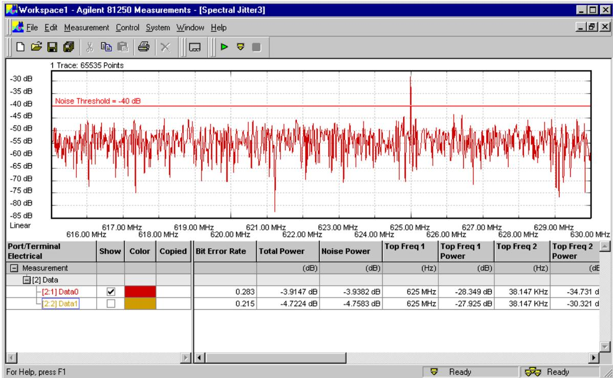
You can see that this jitter component really concentrates on one frequency – 625 MHz.
