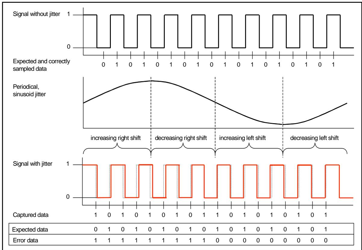
The jitter source moves the received signal to the right and to the left, but the sampling point is fixed (dotted lines show the undisturbed signal). Because we are sampling at the transition point, we get errors when the signal is shifted to the right and no errors when the signal is shifted to the left.
