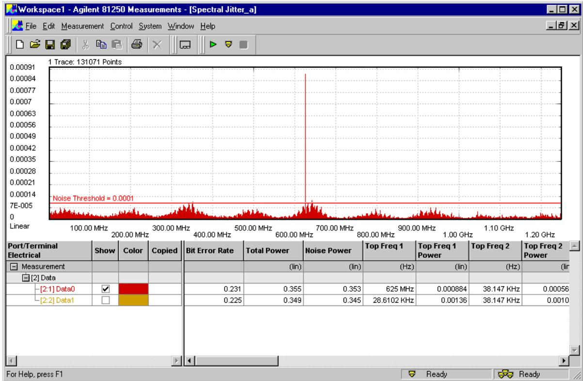
The graph refers to the terminal "Data0". Linear scales are used. A prominent jitter component was found at 625 MHz. It has a power amplitude of 0.000884. Its contribution to the total jitter power of 0.355 is rather small.
