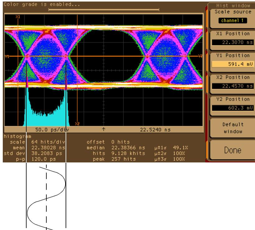
The jitter histogram of a real world signal shows most often a mixture of these characteristic distributions.
