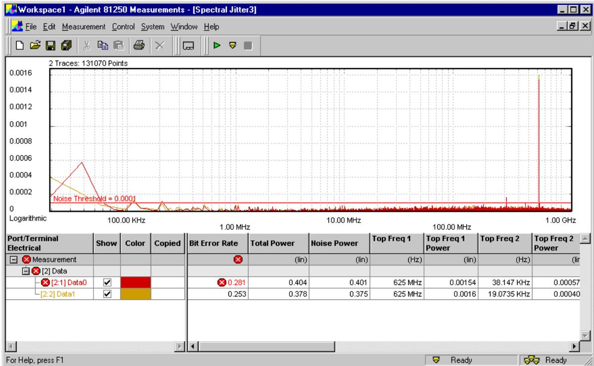
For the next picture, we have defined and enabled two frequency ranges. The power of each range is calculated as the total of all values within the range. We have set the maximum limits to -36 dB.
