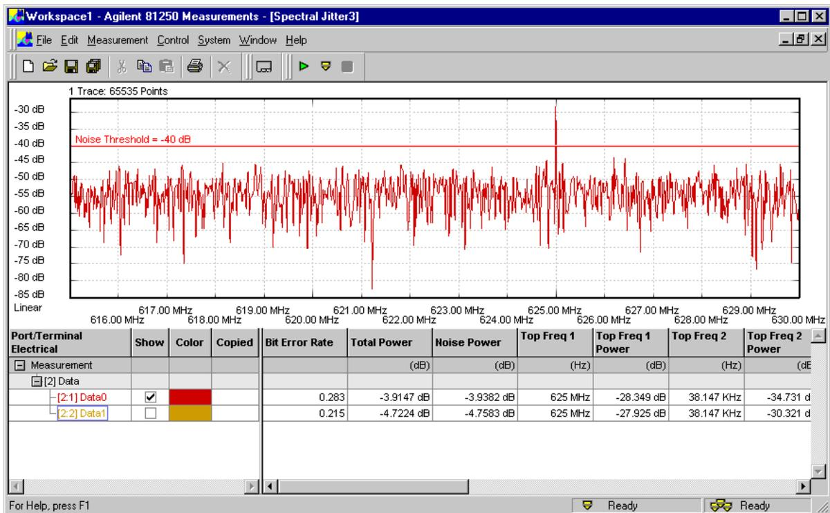
Here, we have defined and enabled a *Zoom range* between 615 MHz and 630 MHz. A linear *Frequency Scale* is used.
