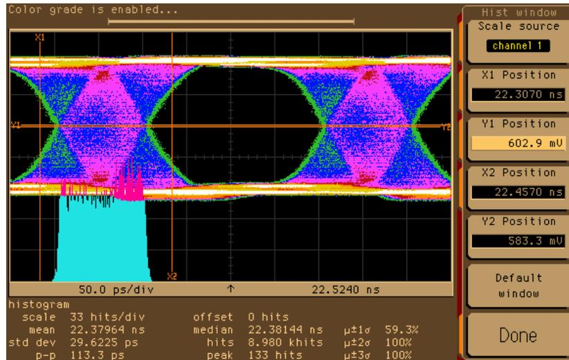
Last, not least, the histogram of jitter modulated by a sinusoid exhibits two significant peaks:
