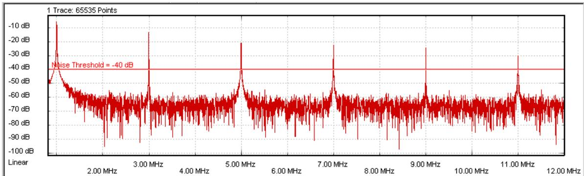
When the repetition period of the characteristic pattern in the error record increases, you will also find the typical sine-x-over-x decay of the spectral power.
