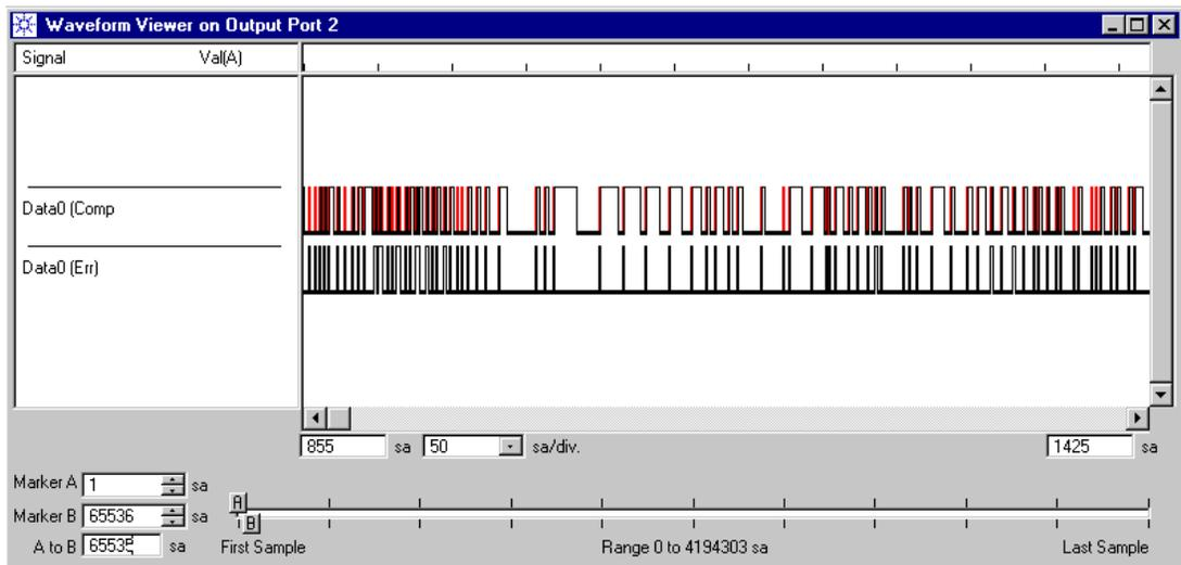
This signal was captured in the jitter region. You can see that the errors are not evenly distributed. The error trace contains patterns that carry spectral information about the jitter.
