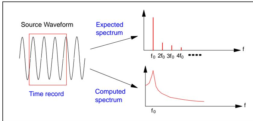
When you perform a Spectral Jitter measurement, it is likely that some degree of leakage occurs. The measurement therefore provides a choice of FFT windows that allow you to detect leakage and to reduce its impact.
