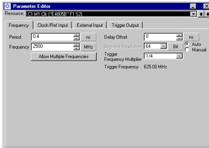
We use a clock rate of 2,500 MHz in this example. This corresponds to a clock period of 0.4 ns.
