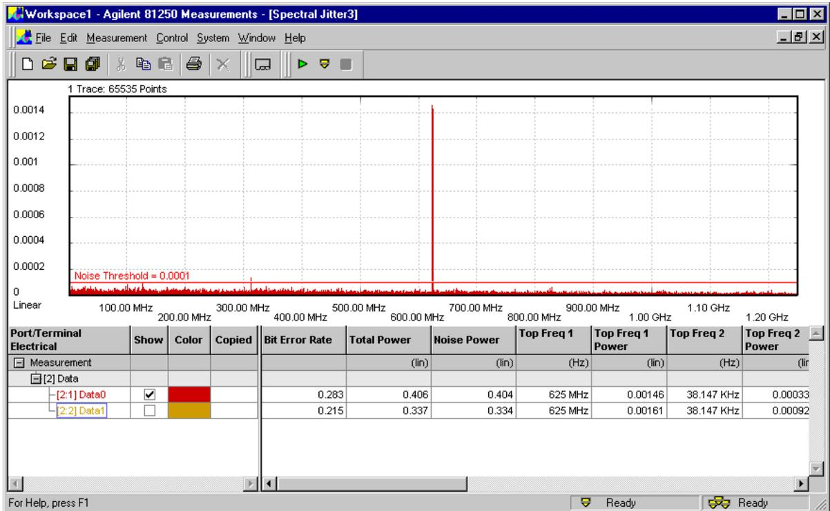
Actually, you see one peak at 625 MHz and not much more. The reason is the linear power scale. A logarithmic power scale has the advantage that you can investigate several decades of the power spectrum in one window.
