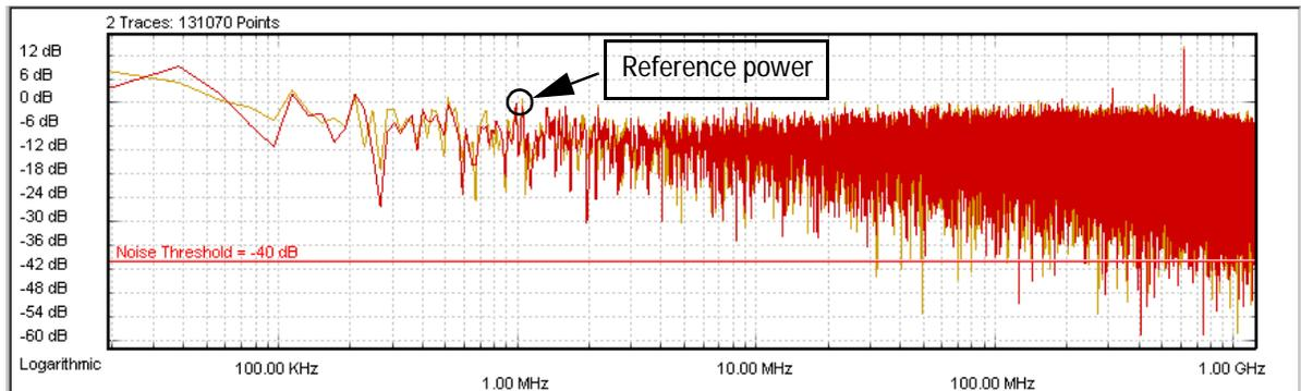
When you set the power values to relative, this changes not only the graphical scale but also the calculated results. You can thus calibrate the power values to any reference.
