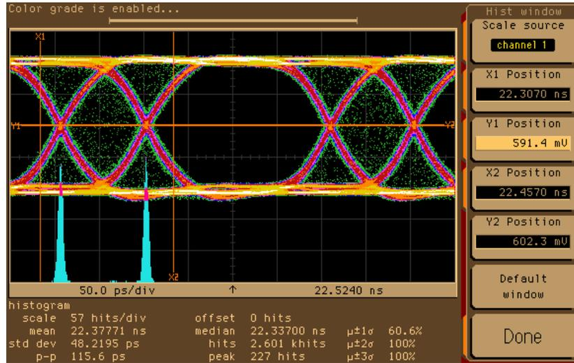
Jitter caused by a triangle signal shows an even distribution:
