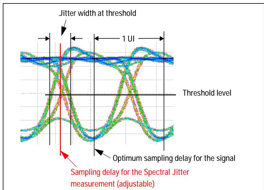
While the measurement is running, correct and incorrect data is captured. The resulting records contain the captured data and the corresponding error information.
