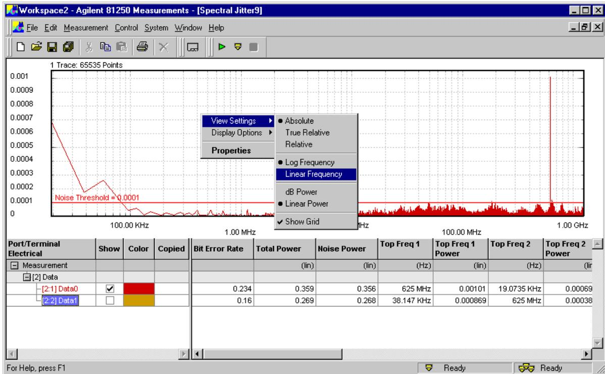
**Frequency scale** A logarithmic frequency scale, as shown in the figure above, allows you to identify low frequency jitter components. A linear scale, as shown in the following figure, hides these peaks.
