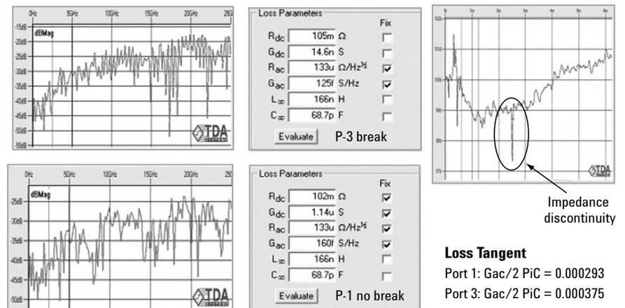
Figure 15. Backplane cable assembly lossy models shows loss tangent with impedance discontinuity due to cable defect on one side of differential pair.
