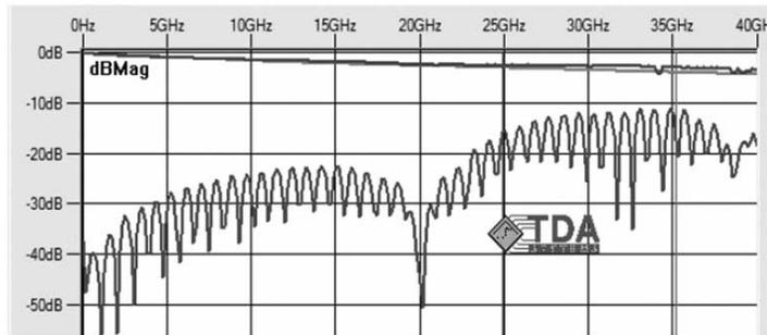
Figure 20. Simulated insertion loss (top) and return loss (bottom) for 30" backplane cable assembly with 112femtoFarad connector.
