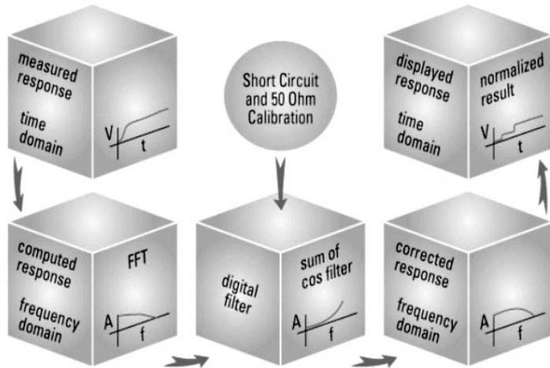
**Figure 8.** Time domain normalization is an error correction technique that resides in firmware inside the TDR oscilloscope. This technique utilizes the Bracewell Transform developed at Stanford University and removes test fixture error by performing frequency domain math functions.
