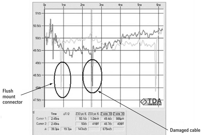
**Figure 16. Impedance discontinuities from two different physical structures can look very similar. However, the intuitive nature of TDR's helps discriminate between a break in the cable and the flush mount connector.**
