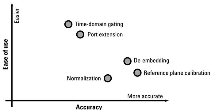
**Figure 7. Various mathematical computations and error correction techniques can be made to enhance measurement accuracy. Usually, ease of use and degree of accuracy are inversely proportional to each other.**
