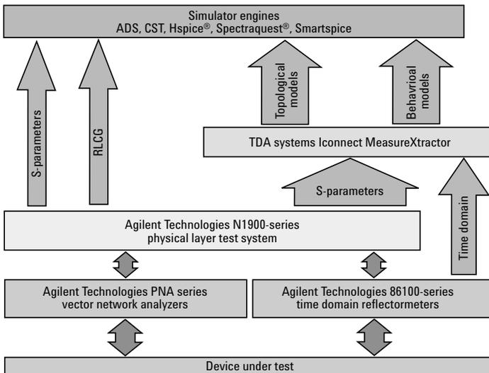
Figure 11. An overview of the many ways to develop models for digital interconnects.
