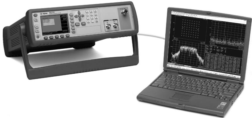
The 89601A/89607A software runs on a PC connected to the N4010A via LAN or USB and provides hardware control, modulation analysis, evaluation, and troubleshooting along with complete results displays. The controls and display of the N4010A are disabled while operating the 89601A/89607A software.
