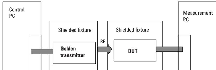
**Figure 11. Using a golden radio for receiver sensitivity testing.**
