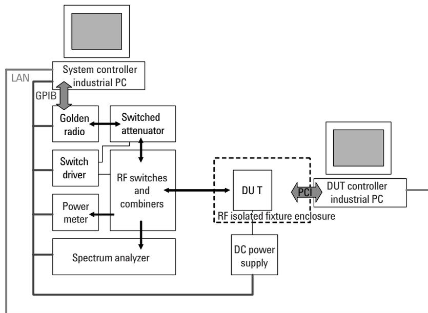
Figure 1. Golden radio-based manufacturing test system.
