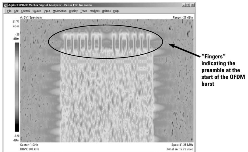
Figure 9. Spectrogram of an OFDM burst.
