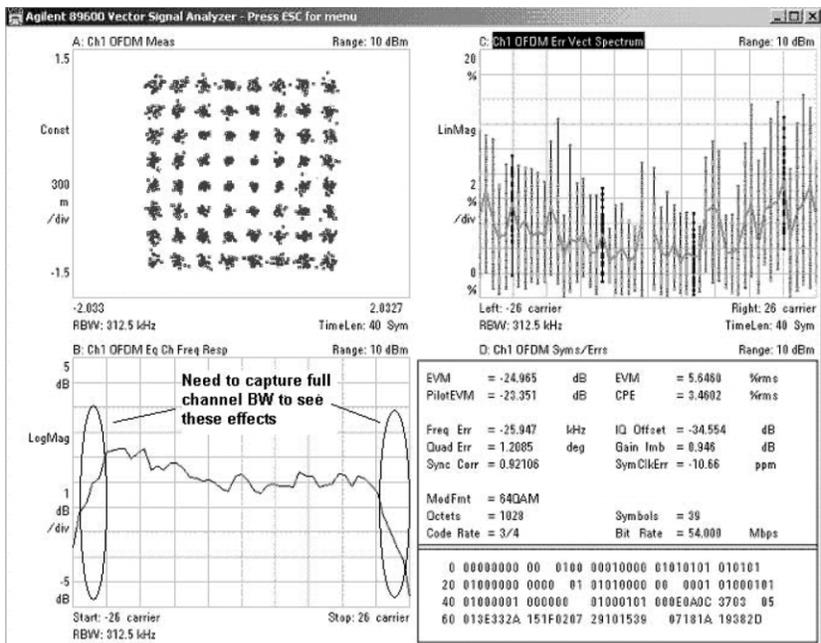
Figure 4. Using full channel bandwidth to measure WLAN.
