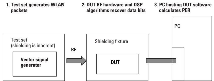
**Figure 12. Using an integrated test set for receiver sensitivity testing.**
