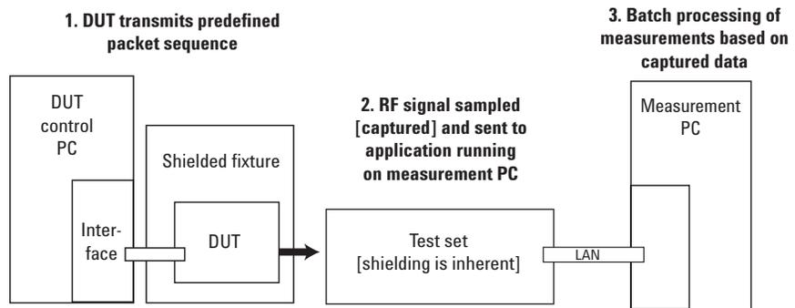
**Figure 7. Measuring transmitter EVM.**
