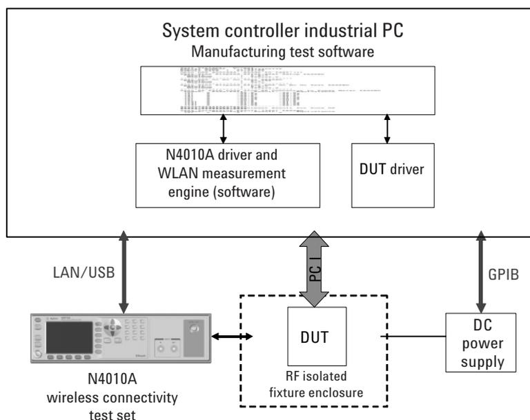
**Figure 3. Integrated WLAN test set manufacturing system.**
