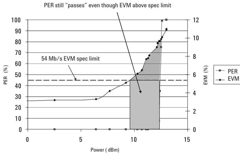
**Figure 8. Characteristics of Tx PER and EVM versus power level from an 802.11g WLAN device.**
