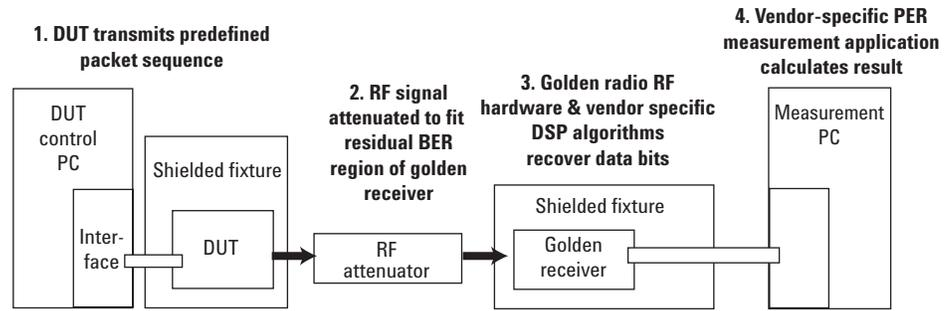
**Figure 6. Measuring transmit packet error rate.**
