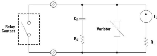
**Figure 11.** *Suppression circuit for limiting surge voltage*
