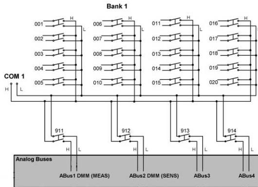
**Figure 10b.** *The Agilent 34980A provides internal busses to expand multiplexer modules without the need for additional Matrix cards. Up to 8 multiplexer cards can be connected to the analog busses.*
