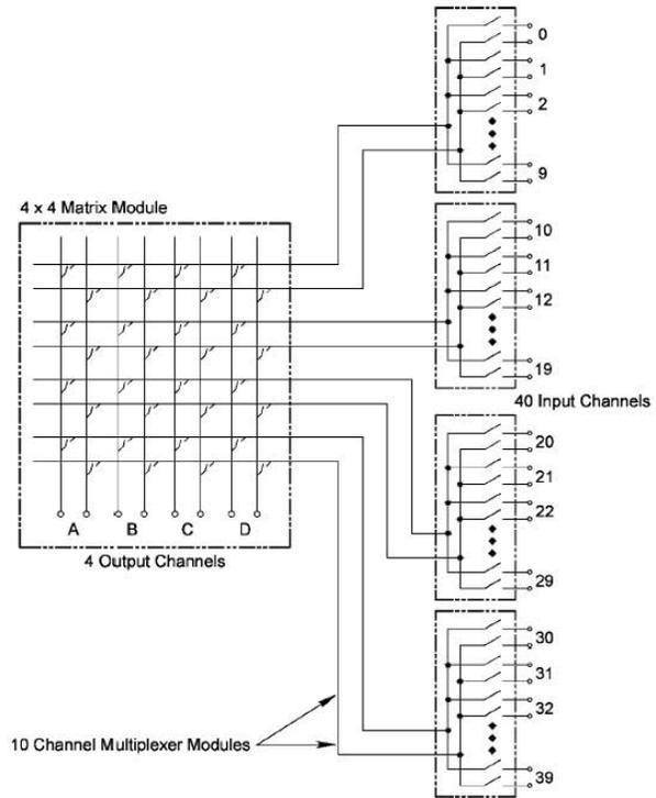
**Figure 10a.** *Multiplexers can be used to effectively and economically expand the number of inputs or outputs of a matrix, although this switching topology does not have the unlimited flexibility of a full crossbar matrix.*
