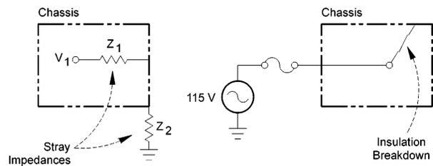
**Figure 20<sup>†</sup>. Instrument chassis should be grounded for safety. Otherwise, it may reach a dangerous voltage level through stray impedances (left) or insulation breakdown (right).**
