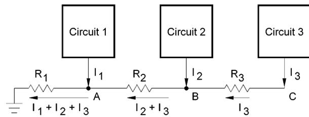
**Figure 22<sup>1</sup>.** Common ground system is a series ground connection and is undesirable from a noise standpoint but has the advantage of simple wiring.
