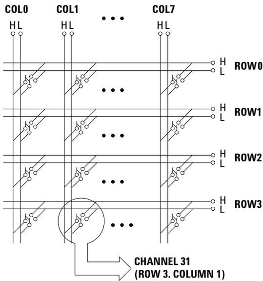
**Figure 8.** A full crossbar matrix, which allows two-wire connection from any point to any point
