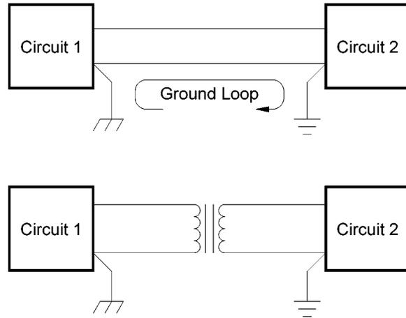
**Figure 28<sup>†</sup>.** A ground loop between two circuits can be broken by inserting an isolation transformer.
