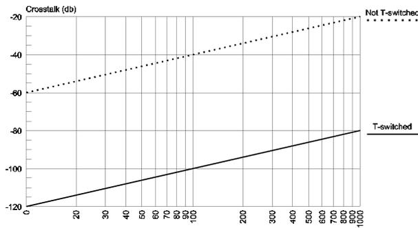
Figure 31. The effect of T-switching on Crosstalk. The effective capacitance between signal paths is minimized to the extent that up to 60 dB of crosstalk isolation is realized through T-switching.
