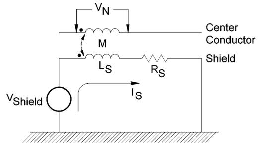
**Figure 18<sup>†</sup>.** Equivalent circuit of shielded conductor.
