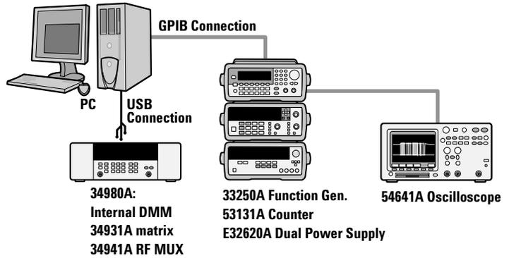
**Figure 32. A typical small testing system consisting of the Agilent 34980A Multifunction Switch/Measure Unit with internal DMM, an oscilloscope, dual power supply, universal counter, and function generator.**
