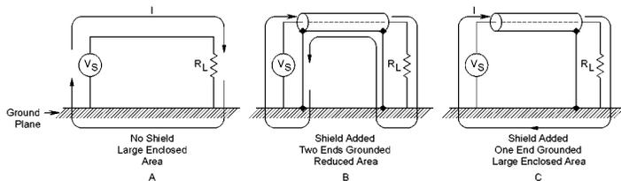
**Figure 19<sup>†</sup>. Effect of shield on receiver loop area.**
