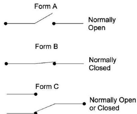
**Figure 2. Simple relay configurations**
