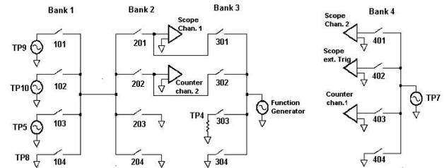
**Figure 33a. The switching topology for the test system consists of 1 quad RF module and 1 matrix module. This represents the RF module used for the AC signals in slot 2.**
