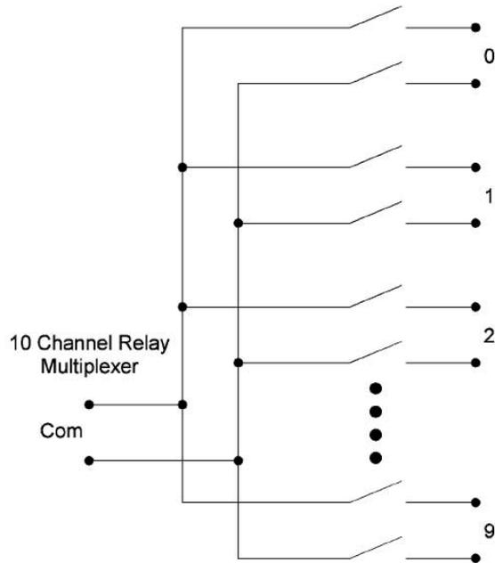
**Figure 5.** A two-wire multiplexing topology. This 10-channel relay multiplexer can be used for floating measurements because both conductors, the signal and the ground return, are connected to the common bus at the same time.
