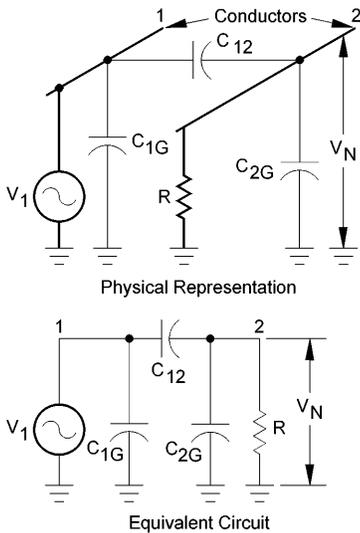
**Figure 14†. Capacitive coupling between two conductors.**
