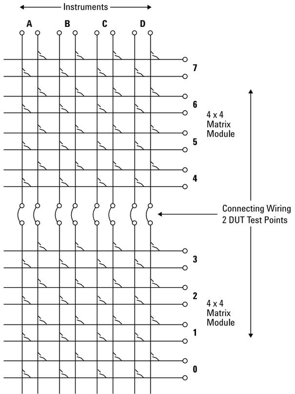
**Figure 9.** An example of connecting multiple matrix cards together to increase the size of the switching system
