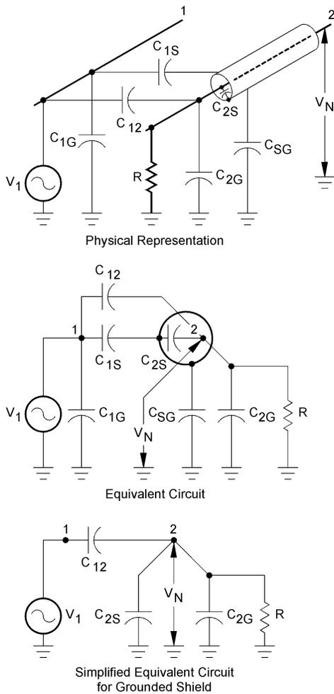
**Figure 17<sup>†</sup>.** Capacitive coupling when receiving conductor has resistance to ground.
