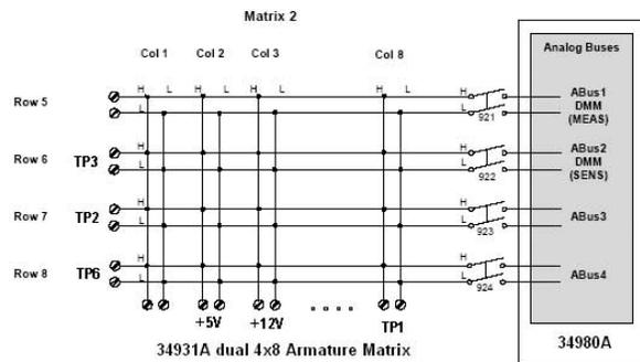
**Figure 33b. The switching topology for the test system consists of 1 quad RF module and 1 matrix module. This represents the Matrix used for low frequency and DC switching. The DMM is internal to the 34980A and connected to row5 to make DC measurements in the Matrix module in slot 1.**
