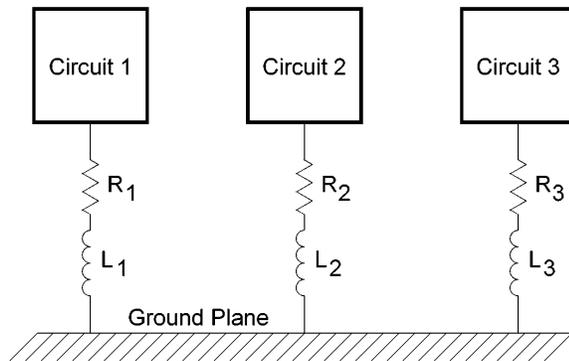
**Figure 24<sup>†</sup>.** Multi-point ground system is a good choice at frequencies above 10 MHz. Impedances  $R_1$ ,  $R_2$ ,  $R_3$ , and  $L_1$  -  $L_3$  should be minimized.
