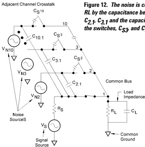
Figure 12. The noise is coupled onto RL by the capacitance between leads  $C_{2,1}$ ,  $C_{3,1}$  and the capacitance across the switches,  $C_{S3}$  and  $C_{S2}$ .
