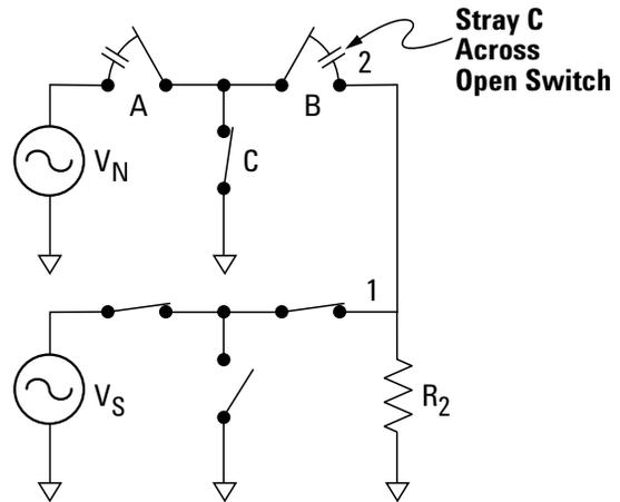
Figure 7. A simplified circuit diagram illustrating T-switching. Conductor 2 is open, so its "C" switch is closed, providing a low-impedance path to ground.
