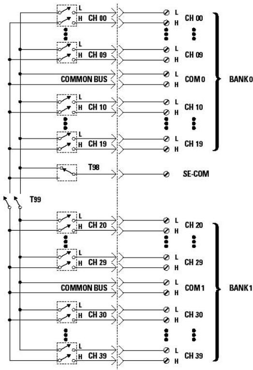
Figure 6. The Agilent N2260A can be configured as an 80-channel 1-wire, 40-channel 2-wire, or 20-channel 4-wire multiplexer.
