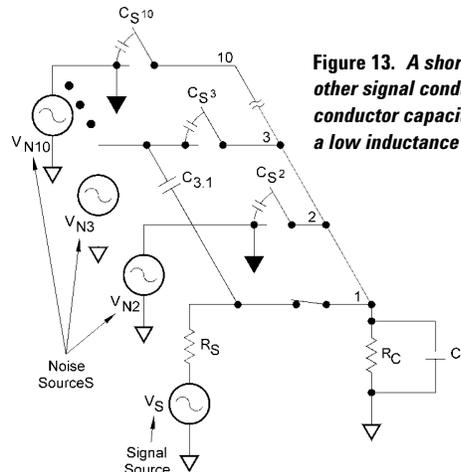
Figure 13. A short placed on every other signal conductor reduces the conductor capacitance and provides a low inductance path to ground.
