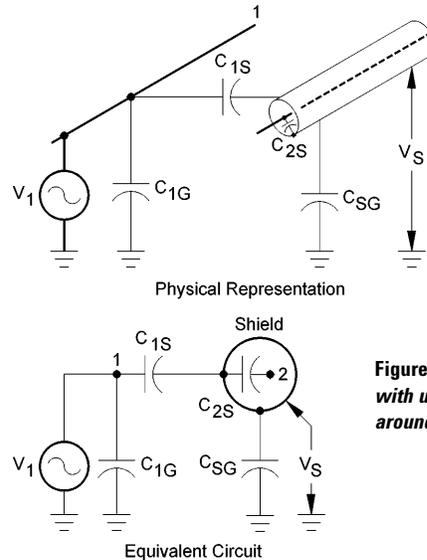
**Figure 16†. Capacitive coupling with unguarded shield placed around receiver conductor.**
