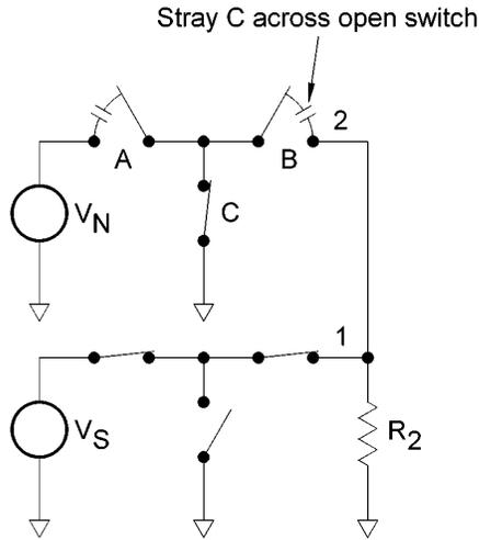
Figure 30. T-Switching.- this is a simplified circuit diagram of how T-switching works. Conductor 2 is open in this diagram; hence, its 'C' switch is closed prodding a low impedance path to ground.
