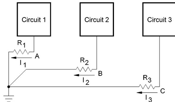
**Figure 23<sup>1</sup>.** Separate ground system is a parallel ground connection and provides good low-frequency grounding, but is mechanically cumbersome.
