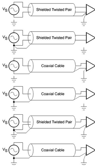
**Figure 27<sup>†</sup>.** Preferred grounded schemes for shielded twisted pairs and coaxial cable at low frequency. The grounds may have large potential differences that can cause ground loops and couple noise into the circuits.
