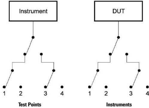
**Figure 3.** A binary switching ladder using form C relays
