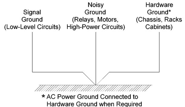
**Figure 25<sup>†</sup>.** These three classes of grounding connections should be kept separate to reduce noise coupling.
