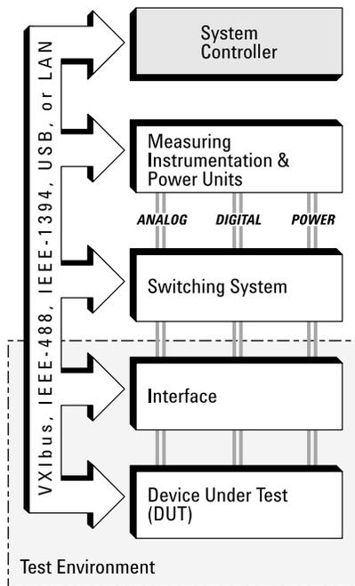
**Figure 1. A generic test-system architecture. Nearly all analog, digital, and power signals pass through the switch subsystem.**
