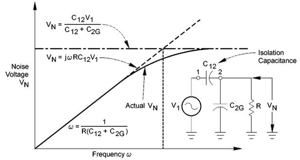
**Figure 15†. Frequency response of capacitive coupled noise voltage.**
