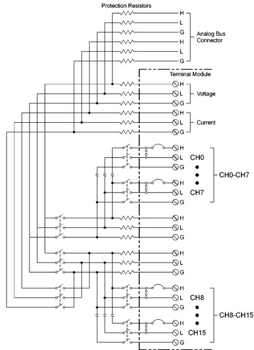
**Figure 29.** 3-Wire multiplexing and tree switching are shown in this illustration of a 20 channel multiplexer card. By placing the tree switch in series with the input channels the effective capacitance of the unused cards in the system is reduced to 1/20th of the normal shunt capacitance in the system. This is very useful for large system configurations.
