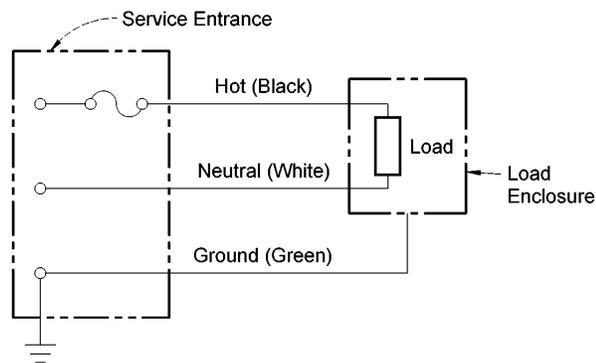
**Figure 21<sup>1</sup>.** Standard 115 V AC power distribution circuit has three leads.
