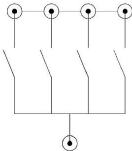
**Figure 4.** A single-ended multiplexing topology used at higher frequencies. Only the signal conductor is switched; the shield is common to all signals.
