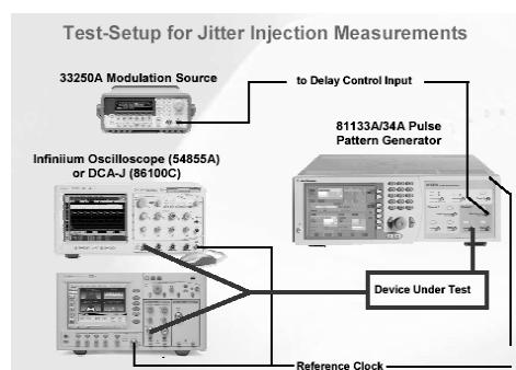
Fig. 4.: Jitter insertion setup
