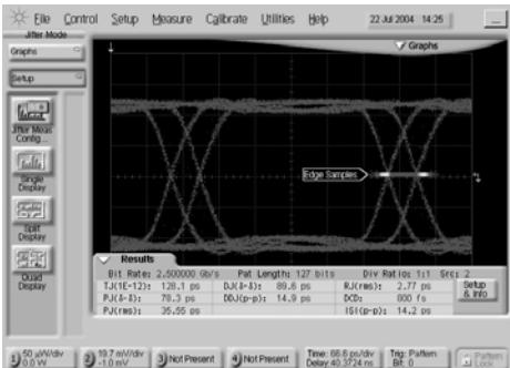
**Fig. 6:** Stressed eye (low-jitter stimulus plus bi-modal jitter) at 2.5 GHz
