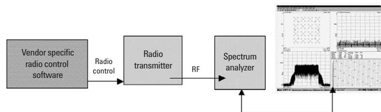
Figure 6. Typical connection diagram for transmitter measurements
