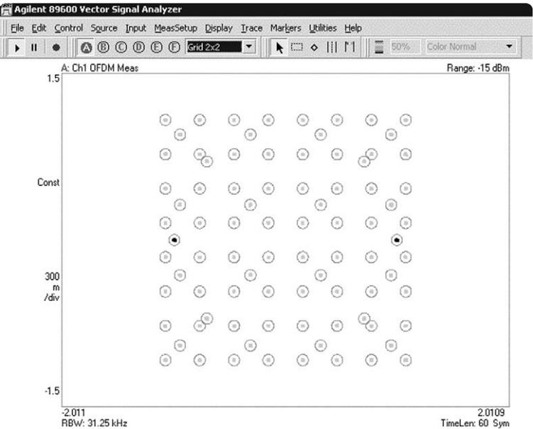
Figure 5. Agilent 89600 IQ measurement of WiMAX downlink frame
