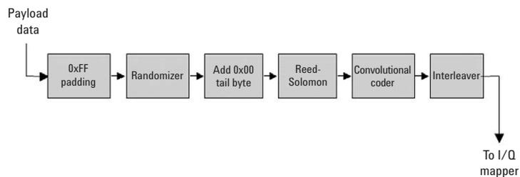
**Figure 4. Channel coding**
