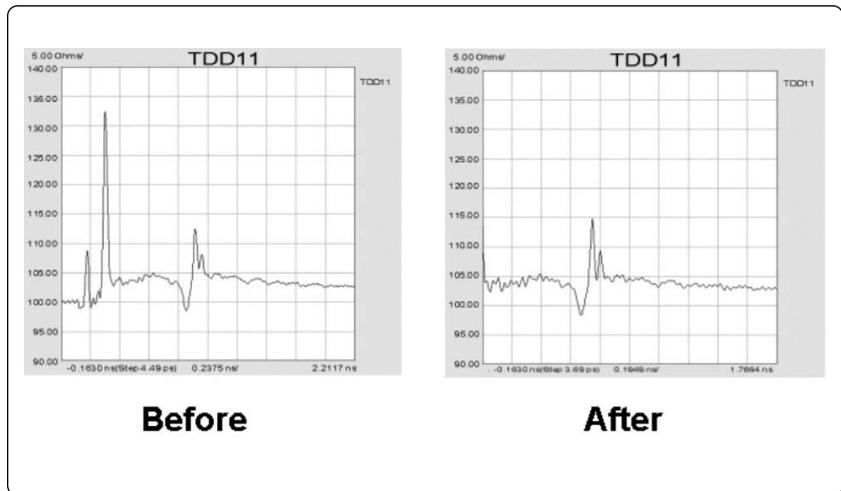
**Figure 20. View of the corrected differential impedance of the FPGA fixture before and after de-embedding.**
