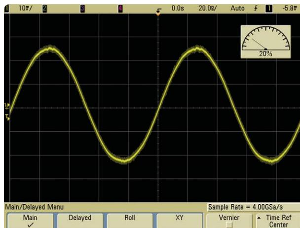
Figure 5. 20% intensity display with 256 levels of intensity gradation
