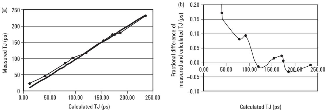
**Figure 7: Comparison of TJ(10<sup>-12</sup>) calculated from the various RJ/DJ calibrations with measurements performed on a BERT. In (a) the measured TJ is plotted against the calculated values, the straight line would correspond to perfect agreement; in (b) the fractional difference between the calculated and measured values of TJ show agreement of better than 10% that can be accounted for by intrinsic uncertainties in the BERTscan technique.**
