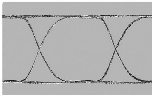
**Figure 3: Comparison of the measured baseline eye diagram, (a), with the eye diagram calculated from the frequency response of the transmission path, time-averaged impulse response of the pattern generator on a PRBS7 and the observed baseline RJ.**
