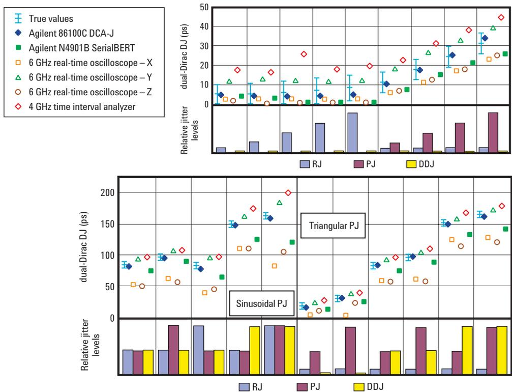
**Figure 8: Measurements of the dual-Dirac DJ with jitter conditions. The jitter conditions (RJ, PJ, DDJ) of each measurement are indicated by the bar graph at the bottom. The true values of dual-Dirac DJ and the calibration uncertainties associated with them are indicated by the left-most, white, data point in each column.**
