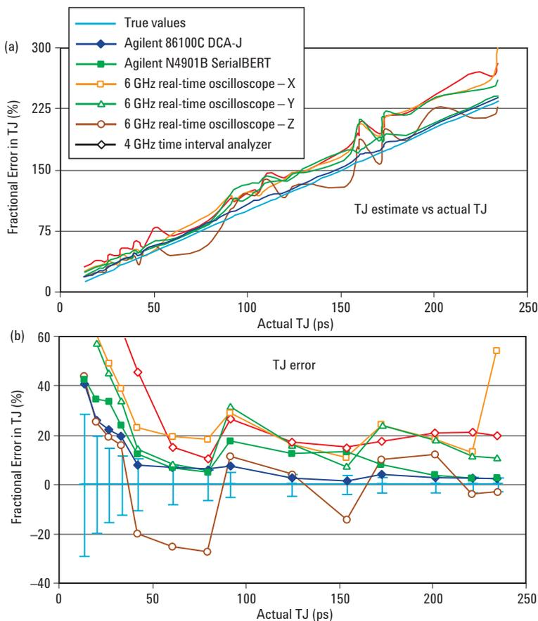
Figure 4: (a)  $TJ(10^{-12})$  estimated by the different test-sets vs the true value (white line), and (b) the percent error in the estimated values – that is, the percent deviation between the estimate and the true value.
