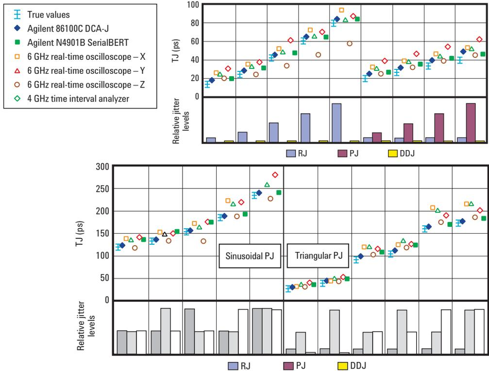
Figure 6: TJ( $10^{-12}$ ) estimates with jitter conditions. The jitter conditions (RJ, PJ, DDJ) of each measurement are indicated by the bar graph at the bottom. The true values of TJ( $10^{-12}$ ) and the calibration uncertainties associated with them are indicated by the left-most, white, data point in each column.
