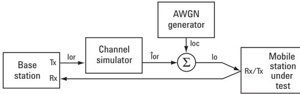
The base station emulator must provide a forward channel with all of the necessary modulation formatting and signaling protocols including code channels with calibrated levels. The channel simulator then adds fading patterns according to user- or standard-defined parameters. Finally, the additive white Gaussian noise (AWGN) generator sums in noise to completely emulate channel conditions under which a mobile station under test may need to operate.
