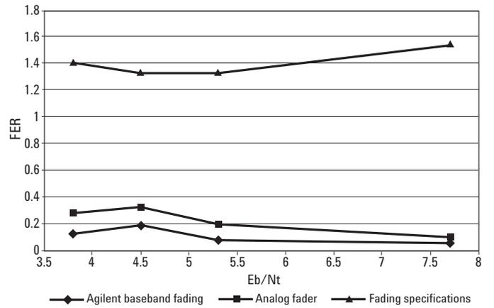
Graph 3: US PCS channel 25 – 30 Km/hr – 1 path – half data rate fading comparison
