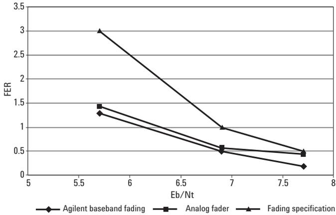
Graph 4: US PCS channel 600 – 30 Km/hr – 1 path – full data rate fading comparison
