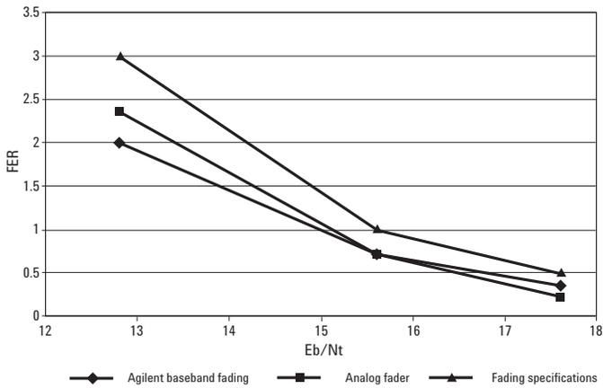
Graph 10: US Cellular channel 1013 – 30 Km/hr – 1 path – eighth data rate fading comparison
