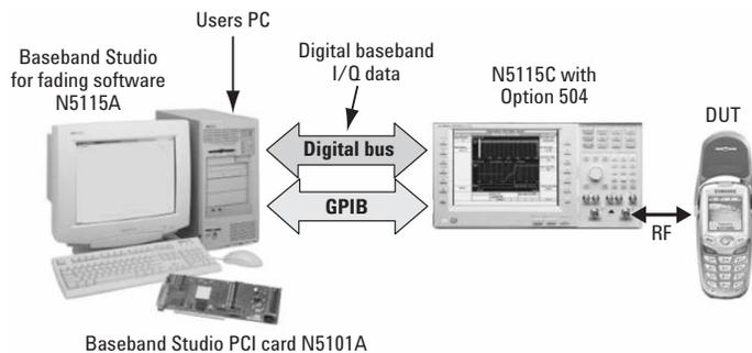
The E5515C transmits accurate, repeatable faded channel signals with minimal effort during setup and operation, and it is priced well below most existing solutions on the market.
