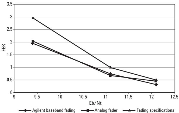
Graph 6: US Cellular channel 384 – 8 Km/hr – 2 path – fading comparison
