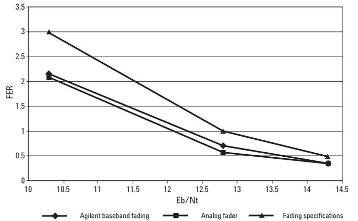
Graph 8: US Cellular channel 384 – 30 Km/hr – 1 path – half data rate fading comparison
