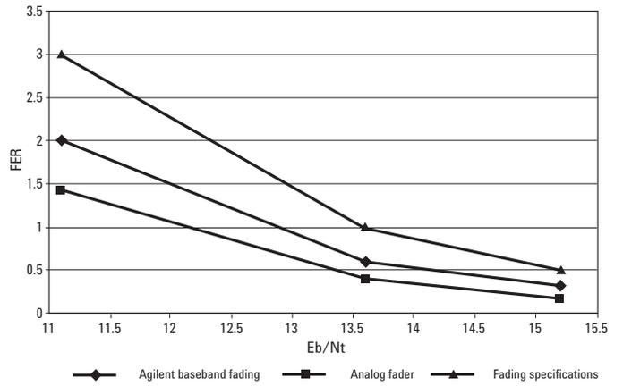
Graph 7: US Cellular channel 384 – 30 Km/hr – 1 path – full data rate fading comparison
