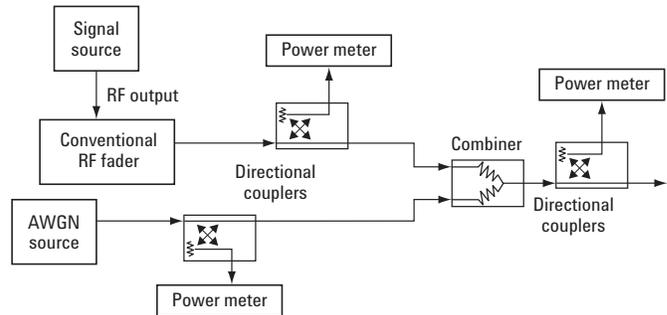
Each setting change can take minutes to measure, adjust, and settle. Consider the time for performing this function multiplied over the length of a fading test plan and the number of devices that can be tested is very limited.
