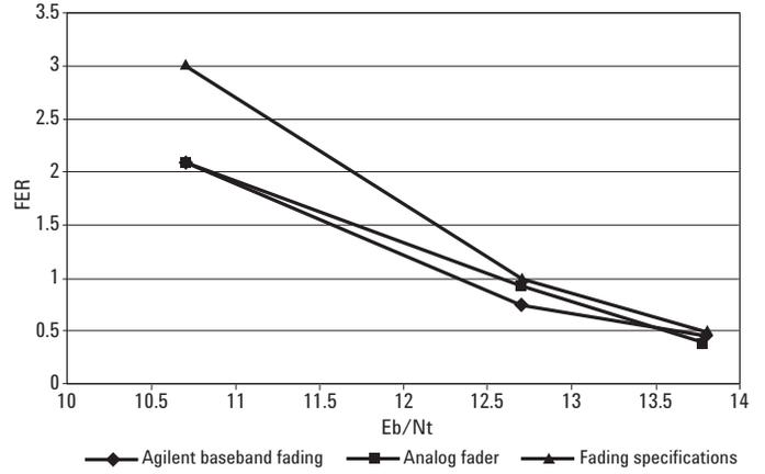
Graph 2: US PCS channel 1175, 30 Km/hr – 1 path – eighth data rate fading comparison
