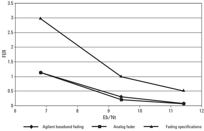
Graph 9: US Cellular channel 384 – 30 Km/hr – 1 path – quarter data rate fading comparison
