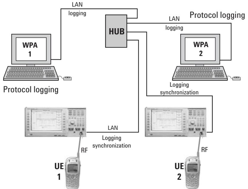
Figure 18. Test configuration for testing UE end-to-end video conferencing capabilities
