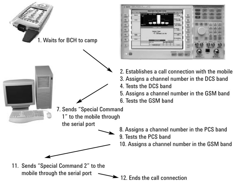
Figure 16. Testing procedure for forcing a band switch
