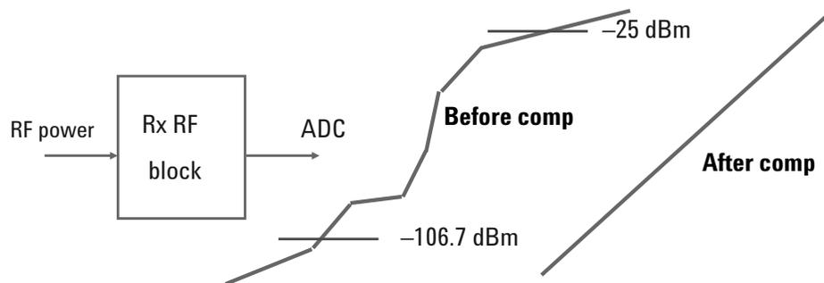
**Figure 7. Model of the Rx of the mobile as a block**
