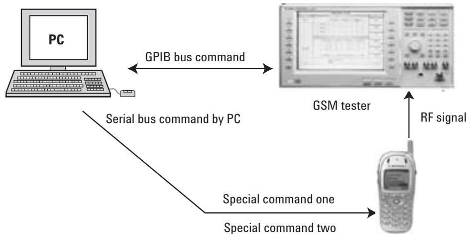
Figure 15. Forcing a band switch using special commands
