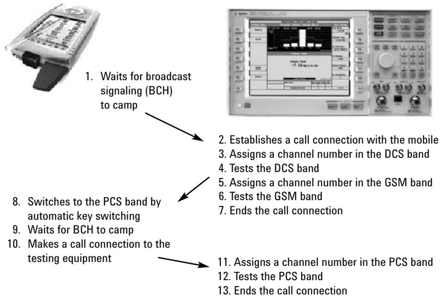
**Figure 13. Traditional method for testing multiple bands**
