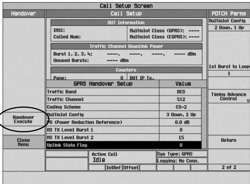
**Figure 17. Simultaneous parameter setting on the 8960 test set saves time**
