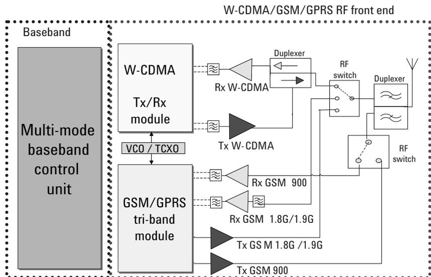
**Figure 3. General multi-mode mobile block diagram**
