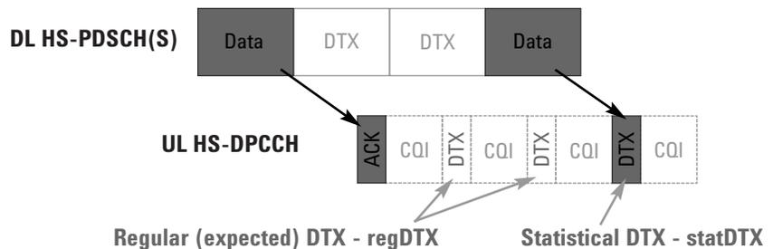
Figure 6. A statDTX is an unexpected DTX response.
