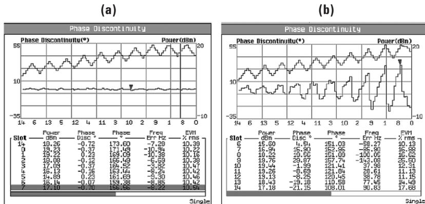
**Figure 14. Measuring phase discontinuity can provide an indication of susceptibility to HS-DPCCH power steps. (a) UE with very stable output phase versus 1 dB power steps, and (b) UE with very poor output phase versus 1 dB power steps.**
