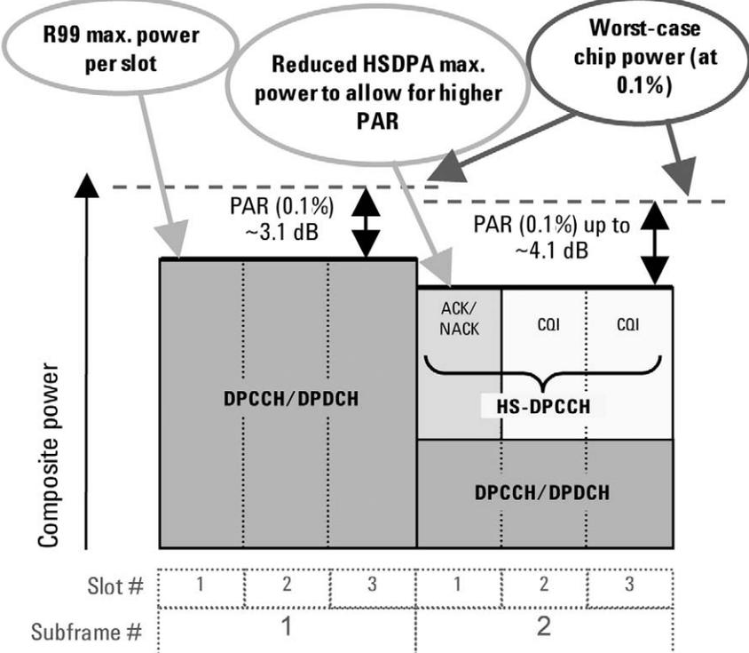
**Figure 1. HS-DPCCH increases uplink peak-to-average power ratio (PAR).**
