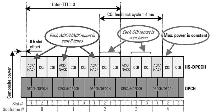
Figure 9. Generic uplink test signal is used for the maximum output power, SEM, and ACLR tests.
