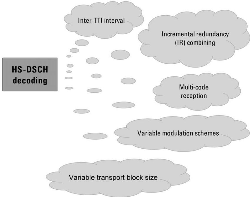
Figure 4. Decoding the downlink HS-DSCH involves complex functionality.
