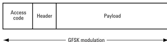
Figure 3. *Bluetooth* basic rate packet format
