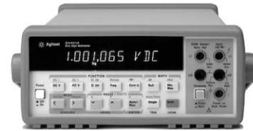
**You configure the 34401A** the same way you configure the 34410A and 34411A. The 34401A uses an analog circuit with a DC blocking capacitor to convert the RMS voltage. The 34401A is specified to measure down to 3 Hz. To make the best possible measurements, select the low frequency filter, use manual ranging, and verify that any DC offset is stable. When you use the slow filter a 7-second delay is inserted to ensure the multimeter is settled.
