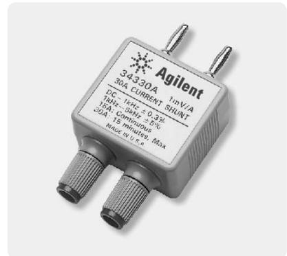
If you want to measure DC and low-frequency AC current (to 30 A, and 15 A continuous) try the Agilent 34330A current shunt, (above) a precision 0.001-ohm resistor housed in a plastic case surrounded by epoxy. Output is 1mV per A of current passing through the shunt. The current to be measured is connected to the shunt via binding posts. Simply inset the wire and tighten the binding post for easy connections.
