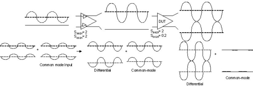
**Figure 14.** A limiting amplifier driven by a true-differential-mode signal does not show compression
