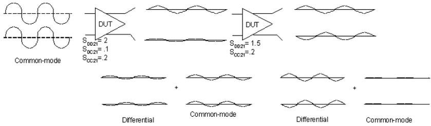
**Figure 12.** Here we drive the amplifier with a true-common-mode signal. Since the first stage suppresses the common-mode, there is very little signal to drive the output stage so no compression occurs
