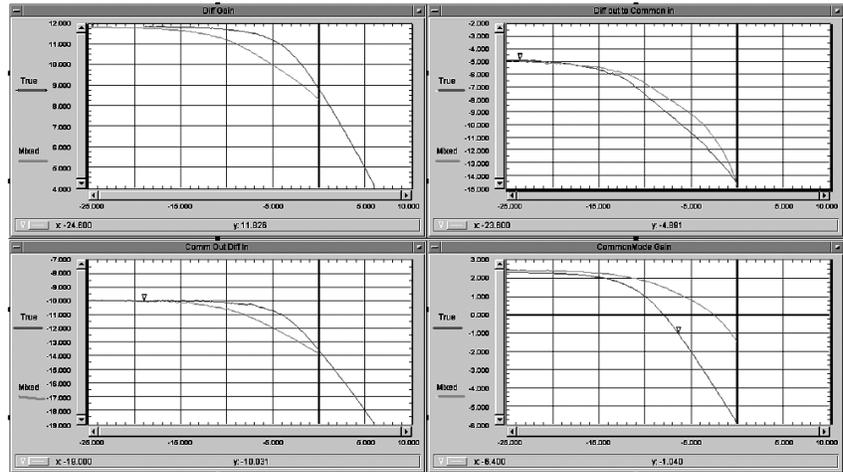
**Figure 6. Mixed-mode and true-mode measurements of a limiting non-linear amplifier – Note the differential gain SDD21 is not the same when measured with a true-mode signal as compared with a single-ended mixed mode measurement**
