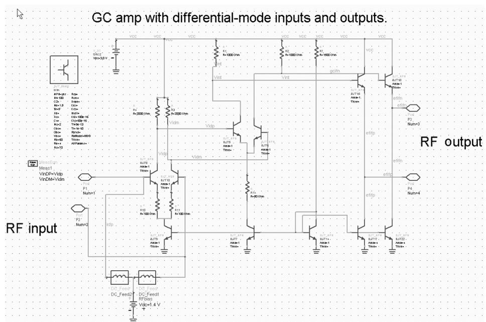
Figure 15. Gilbert-cell differential amplifier used in simulations
