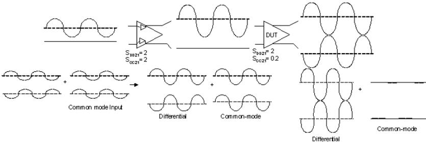
**Figure 13.** The first stage of this amplifier does not have common mode suppression, though the second stage does. Here input stage compresses on the positive half-cycles. Note that the single-ended signal causes compression, for a given nominal differential output voltage
