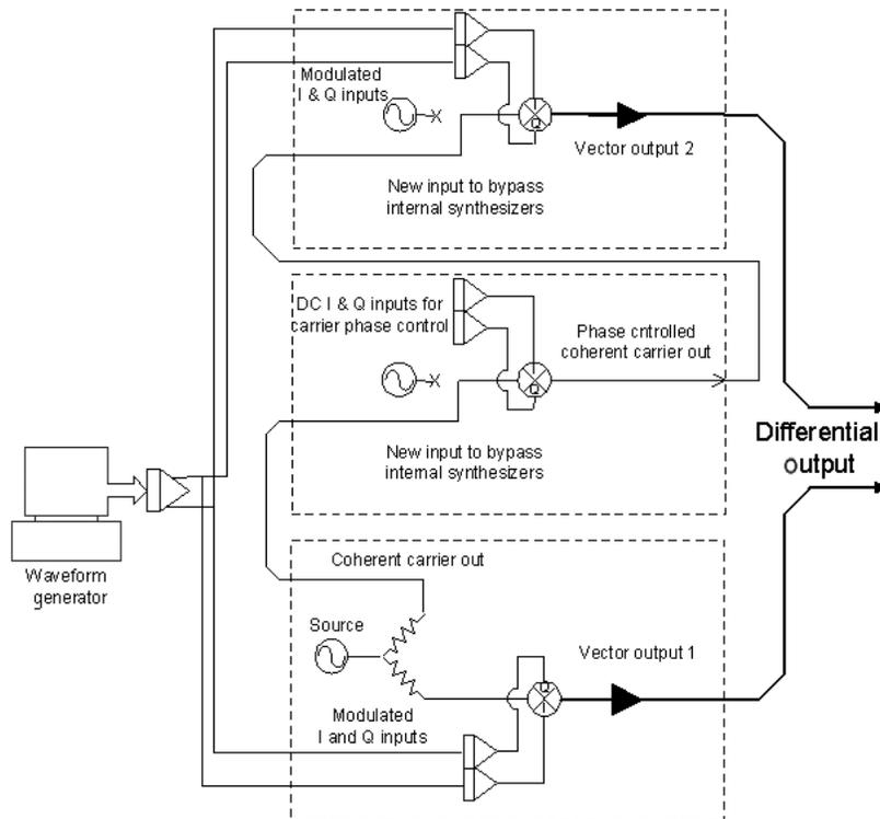
Figure 1. Block diagram for generating balanced modulated signals
