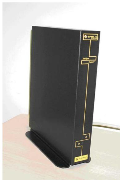
Figure 3: The Agilent Instrument Controller is a network device used by Agilent OL to connect all instruments into the software framework. It has a small footprint, approximately the size of a laptop, and can connect up to 4 different instruments and it supports a variety of different communication protocols (RS232, IEEE, SCSI, Ethernet, USB).
