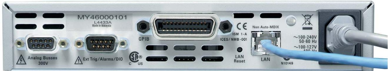
**Figure 3.** Rear panel of Agilent L4433A showing LAN cable. This inexpensive cable connects directly to many PCs or networks without the need to install an I/O card
