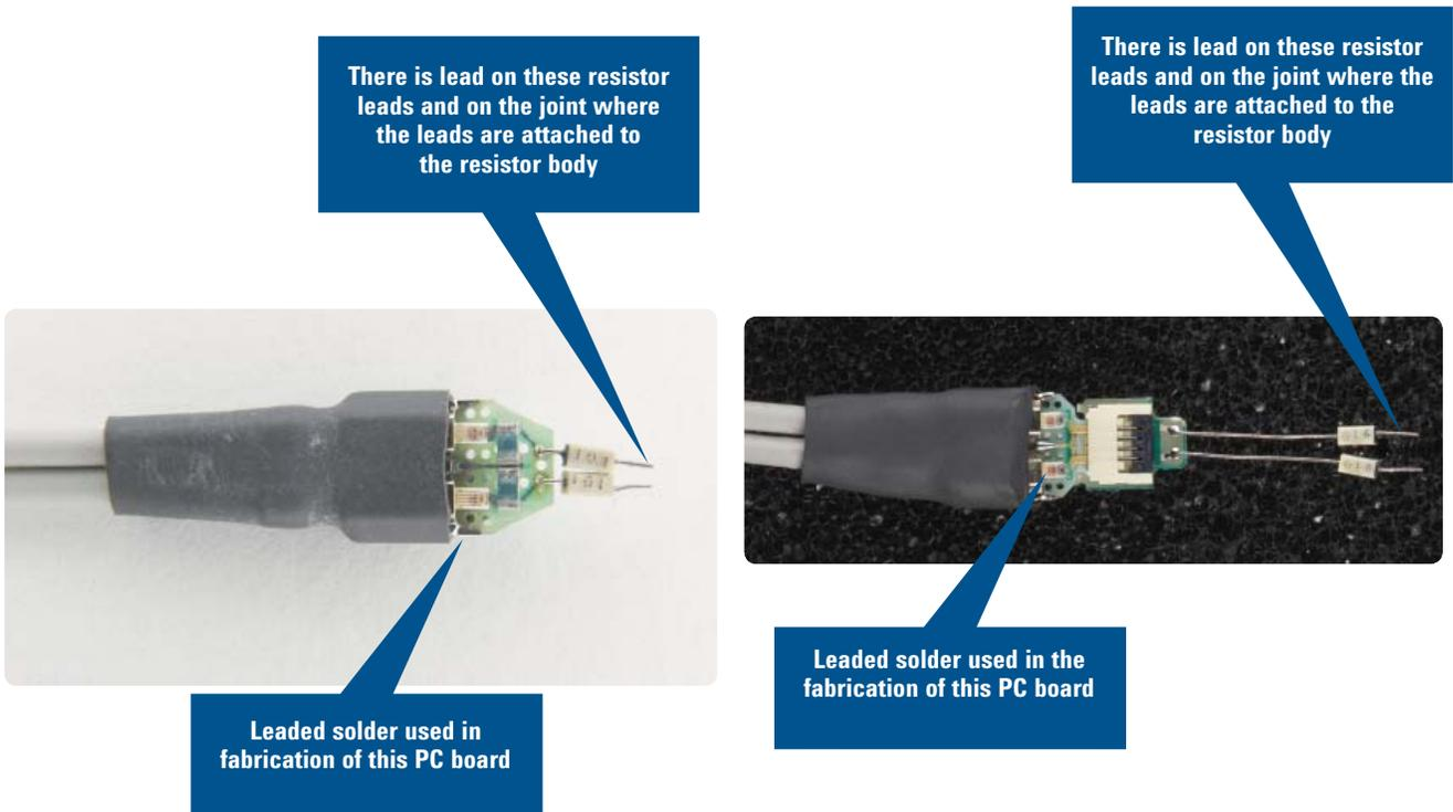
Figure 2. E2677A 8-GHz solder-in InfiniMax probe head
