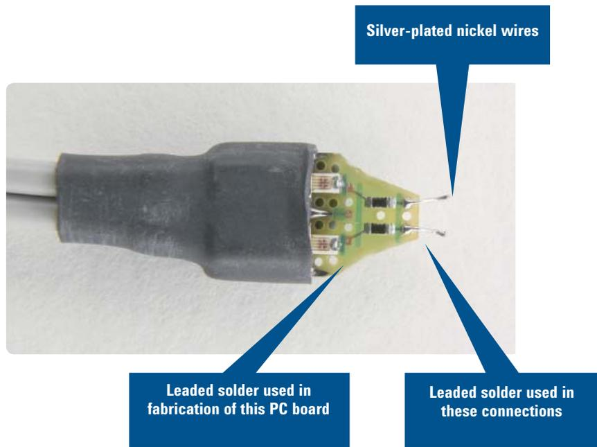
Figure 1. N5381A 12-GHz InfiniiMax solder-in probe head
