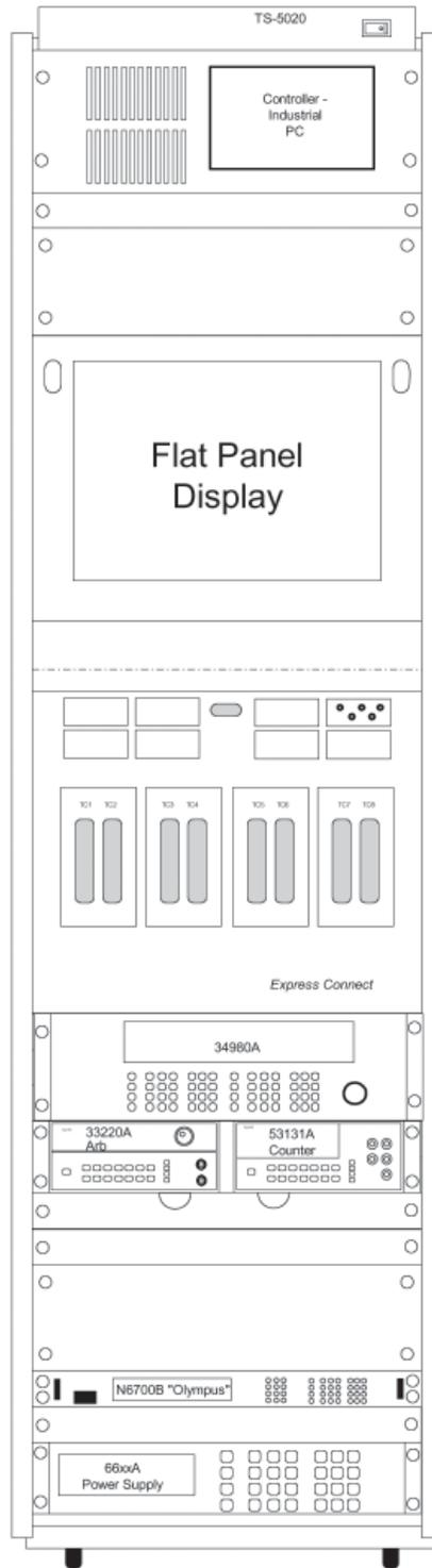
Figure 3: Agilent TS-5020 Automotive Functional Test System
