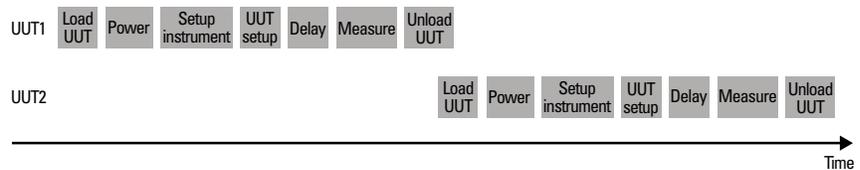
Figure 6: Single-up testing of two or more UUTs
