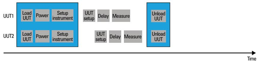
Figure 7: Multi-up testing of two or more UUTs
