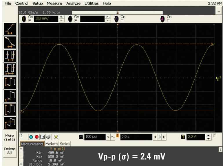
Figure 12a: 2.5-GHz sine wave captured on the Agilent Infiniium oscilloscope sampling at 20 GSa/s (non-interleaved)
