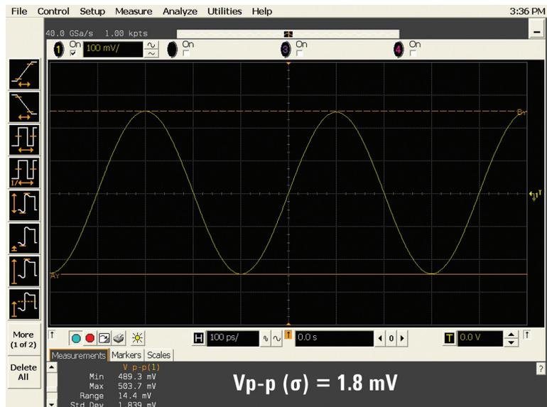
Figure 12b: 2.5-GHz sine wave captured on the Agilent Infiniium oscilloscope sampling at 40 GSa/s (interleaved)
