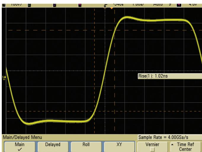
**Figure 7: Agilent 500-MHz bandwidth scope sampling at 4 GSa/s produces minimal measurement improvement over sampling at 2 GSa/s**
