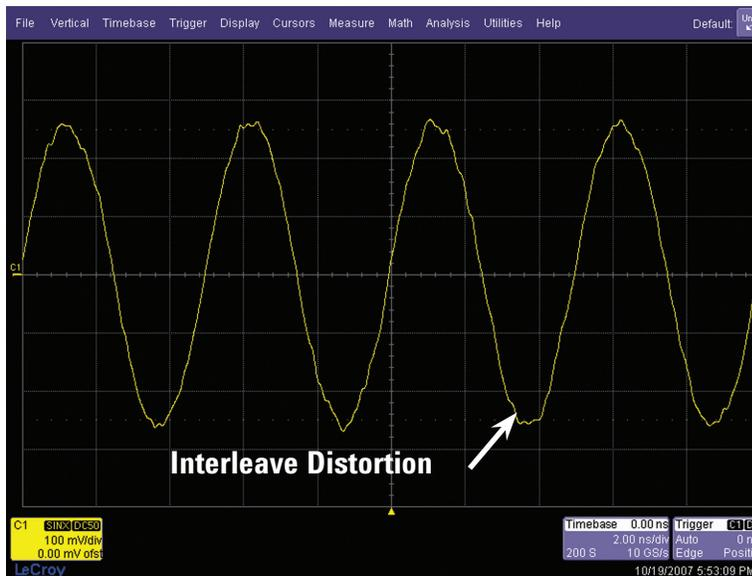
Figure 11b: 200-MHz sine wave captured on a LeCroy 1-GHz bandwidth oscilloscope sampling at 10 GSa/s
