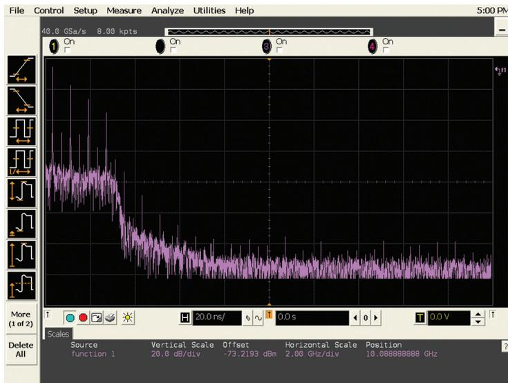
Figure 16a: FFT analysis on a 400-MHz clock using an Agilent Infiniium 3-GHz bandwidth oscilloscope
