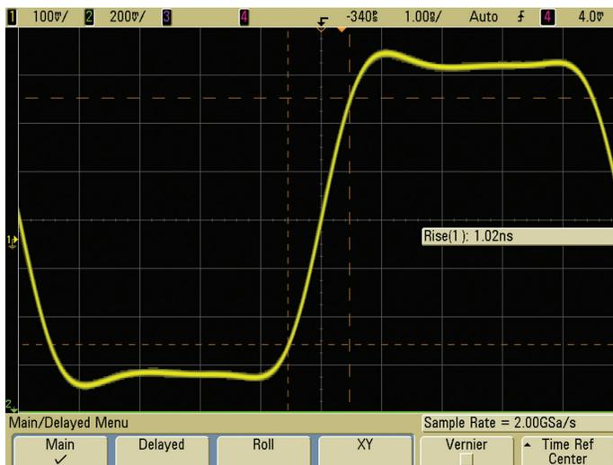
**Figure 6: Agilent 500-MHz bandwidth scope sampling at 2 GSa/s shows an accurate measurement of this 100-MHz clock with a 1-ns edge speed**
