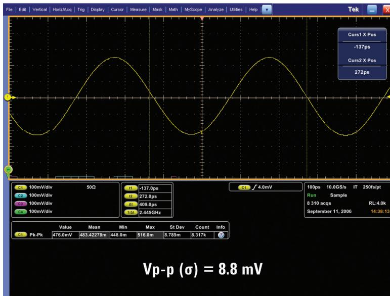
Figure 13a: 2.5-GHz sine wave captured on a Tektronix 2.5-GHz bandwidth oscilloscope sampling at 10 GSa/s (non-interleaved)
