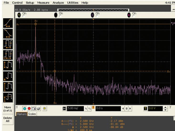
Figure 14a: FFT analysis of 2.5-GHz sine wave captured on an Agilent Infiniium oscilloscope sampling at 40 GSa/s
