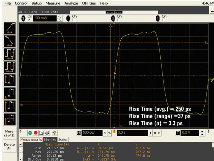
Figure 15a: 400-MHz clock captured on an Agilent Infiniium 3-GHz oscilloscope sampling at 40 GSa/s
