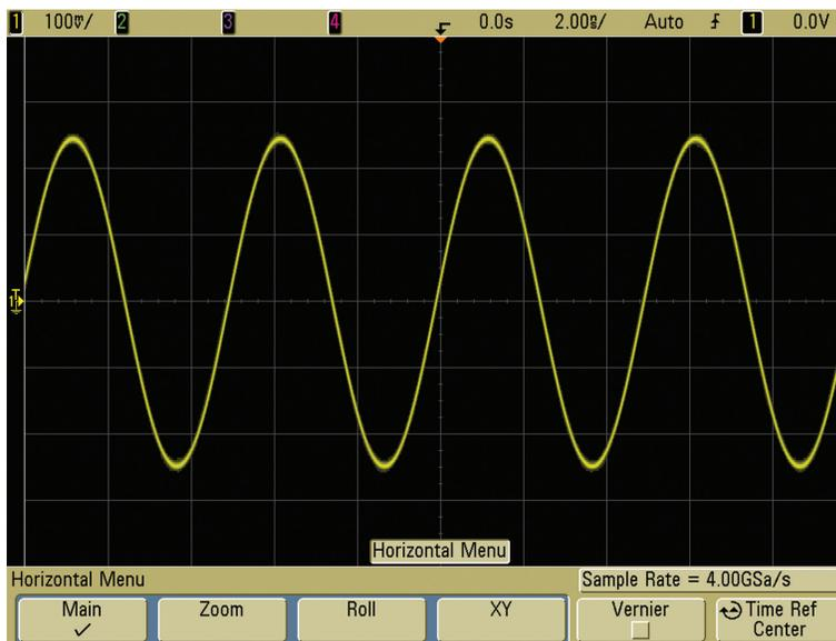
Figure 11a: 200-MHz sine wave captured on an Agilent 1-GHz bandwidth oscilloscope sampling at 4 GSa/s
