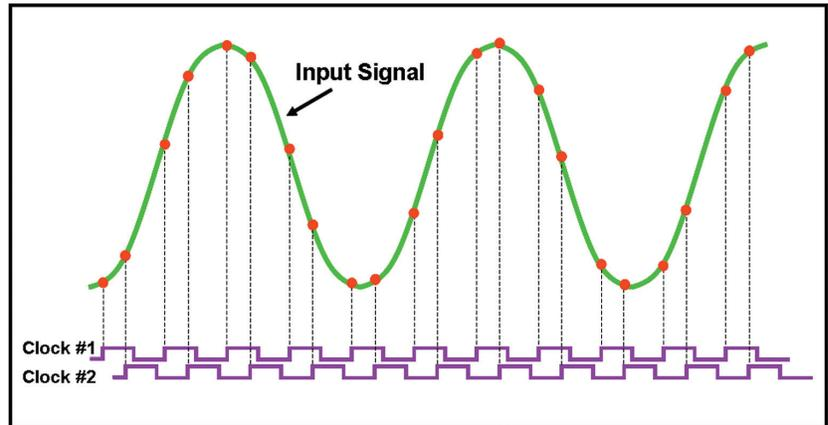
Figure 9: Timing diagram showing non-evenly spaced samples
