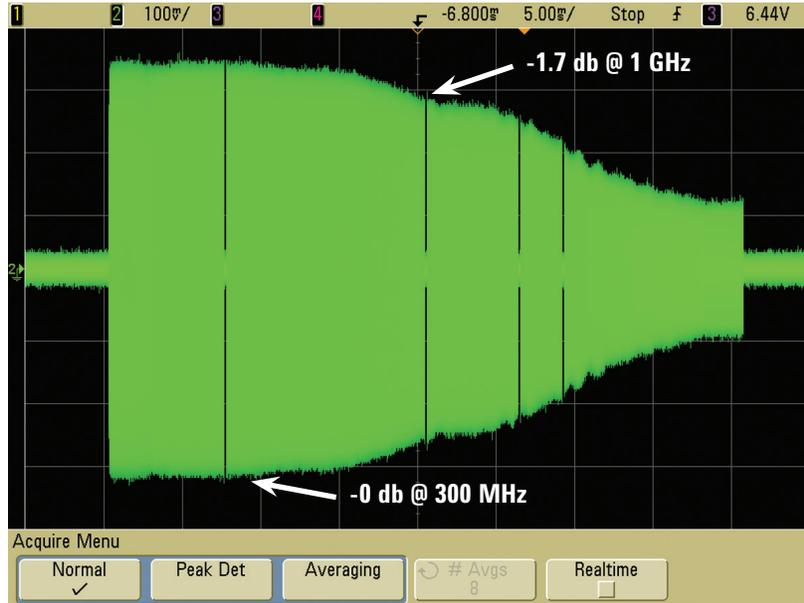
Figure 7: Swept frequency response test on Agilent's MS07104B 1-GHz bandwidth scope
