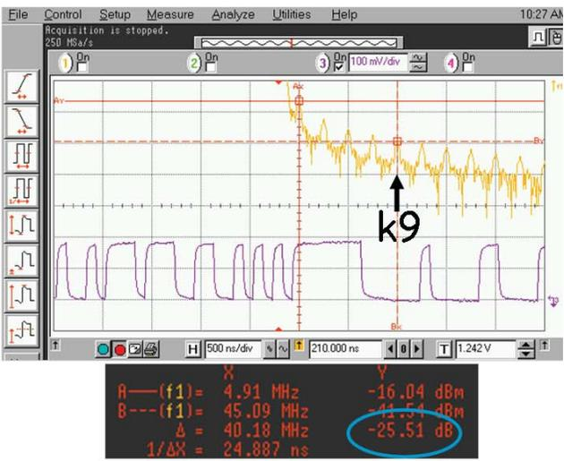
Figure 25: Spectral view of the signal at the end of the cable, the harmonic K9 is reduced by 6.2 dB.
