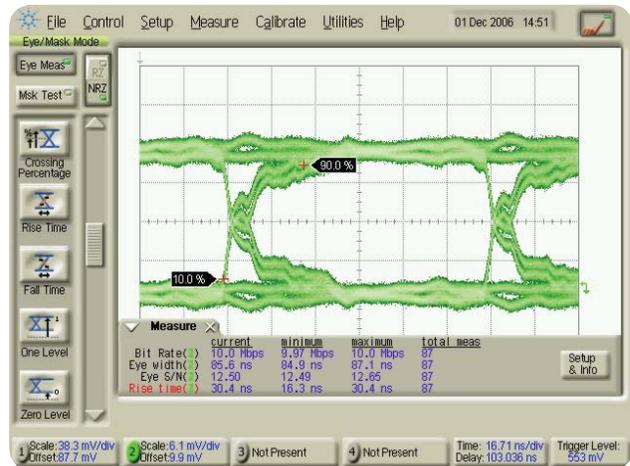
Figure 21: Signal measurement at 10 Mb/s with six 1 m stubs, measured at the un-terminated end of a stub.
