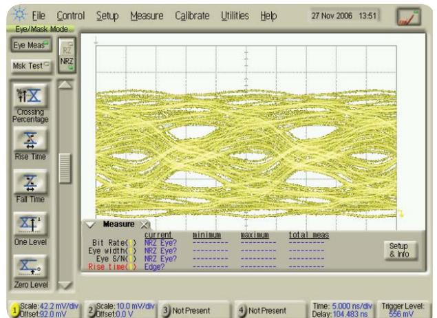
Figure 28: Signal measurement at 50 Mb/s at terminated end of cable with 6 stubs added
