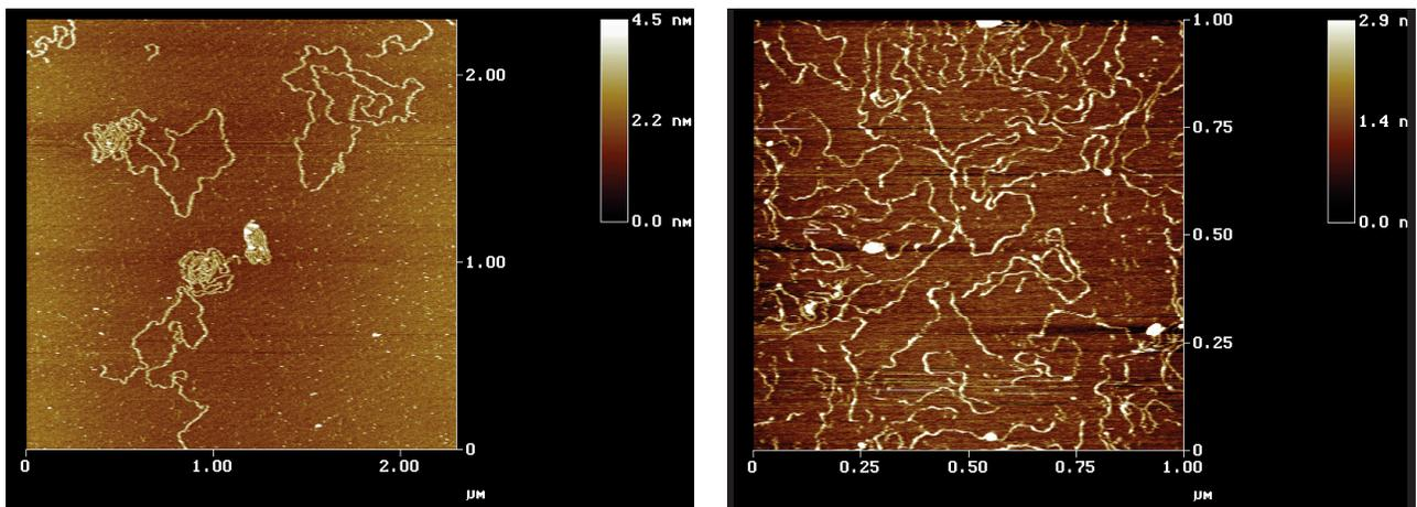
**Figure 3.** Two images of plasmid DNA molecules adsorbed on freshly cleaved mica surfaces in 1-mM  $MgCl_2$  solutions. The measurements were taken with single carbon nanotube AFM tips under MAC Mode control.
