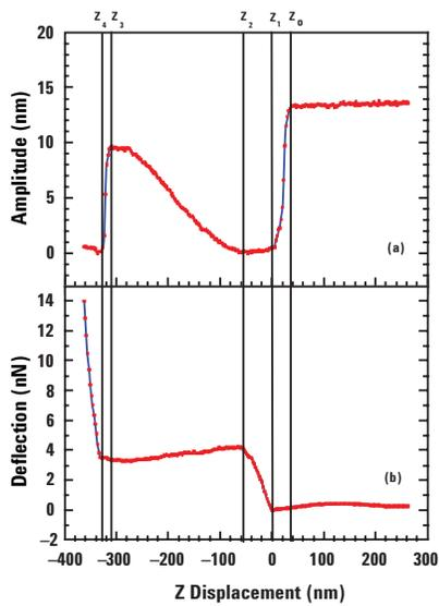
**Figure 1.** The change of the (a) AC oscillation amplitude and (b) DC deflection signal of the cantilever vs. the sample surface-tip distance. The cantilever was prepared with carbon nanotubes at the tip and magnetic films coated at the back. The measurements were carried out on a freshly cleaved mica surface under double deionized water. The cantilever oscillation was driven by a MAC Mode module at 30 kHz.
