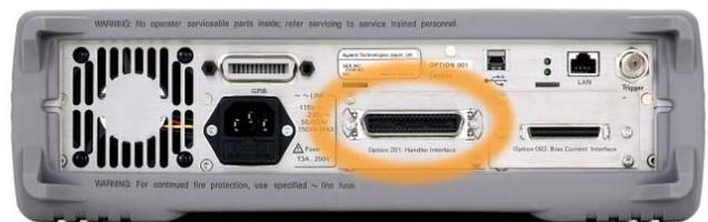
Figure 6. Scanner interface of multiple device testing
