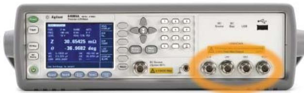
Figure 5. Test ports of the E4980A
