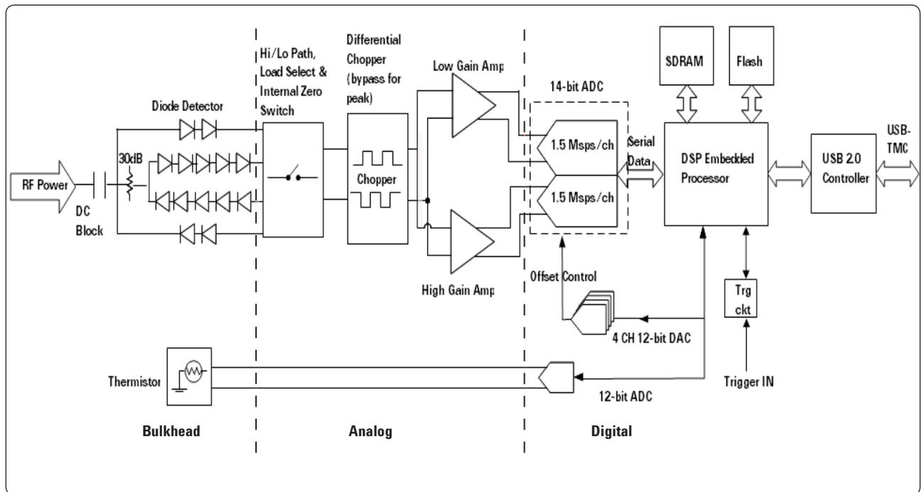
Figure 6 U2000 Series block diagram, showing the internal processing of power data. The diode stacks are shown abbreviated graphically, the actual low power path has 2-diode balanced stacks and the high power path has 5-diode stacks.
