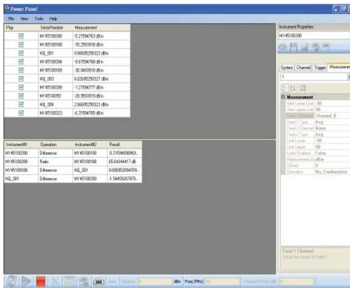
Figure 5 Multiple U2000 Series sensors in multi-list view.
