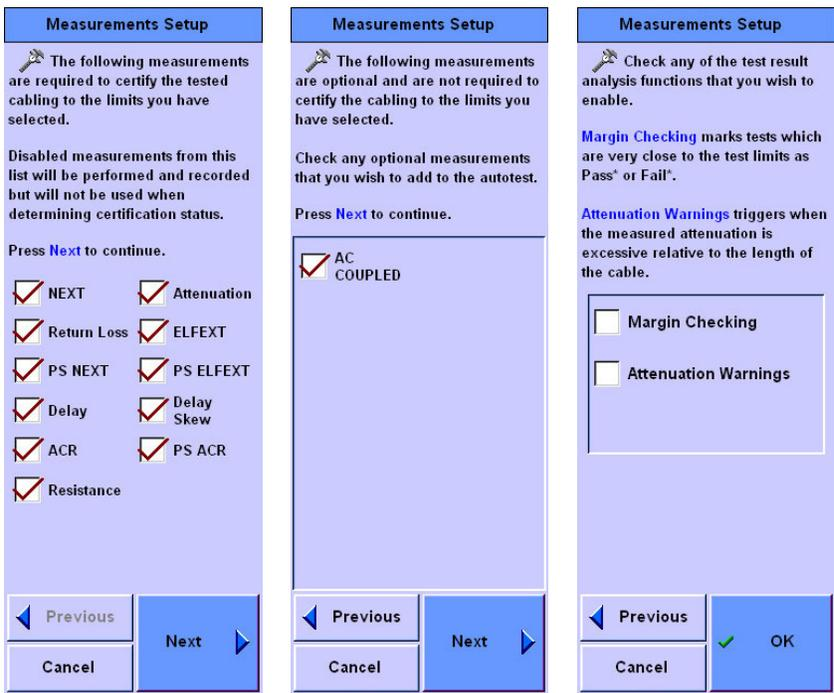
Figure 6 Enabling AC Coupled Testing
