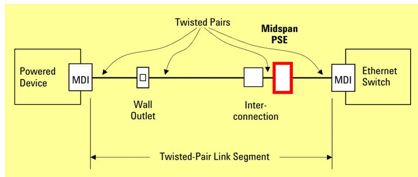
Figure 2 Powering the Inserted Midspan
