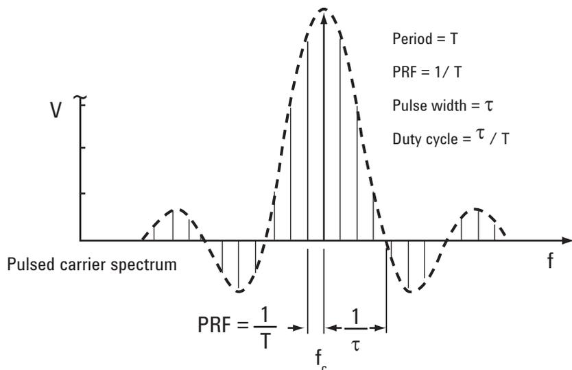
Figure 14. Pulsed spectrum
