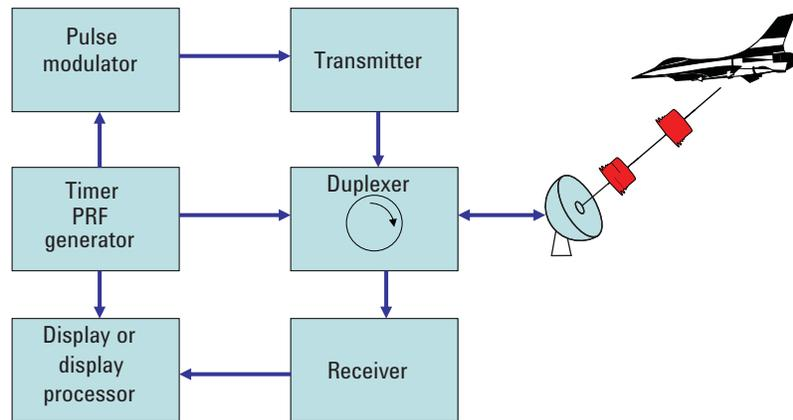
**Figure 4. Basic radar block diagram**
