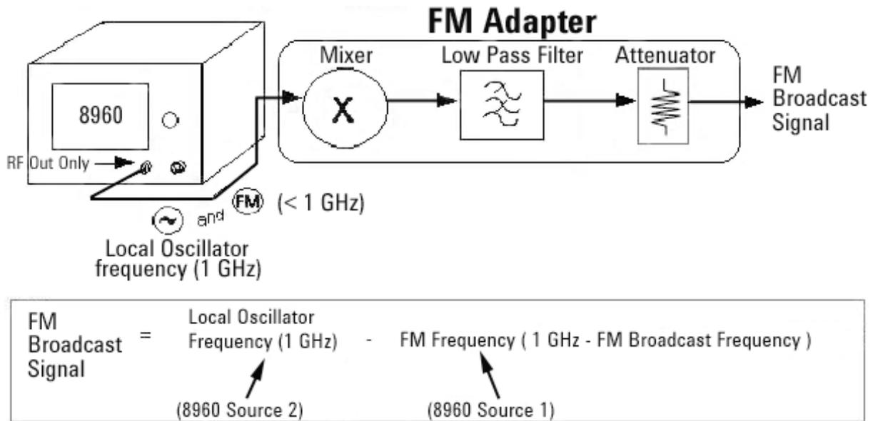
Figure 1. Simplified block diagram of how the system generates the FM Broadcast Signal.
