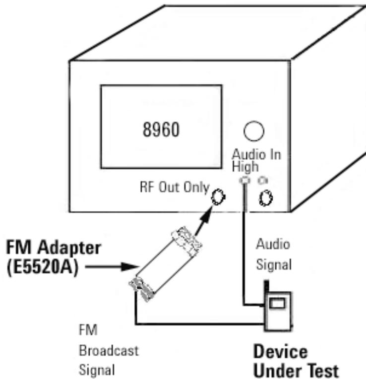
Figure 3. 8960 Series 10 Wireless Communications Test Set, FM Adapter, and DUT setup for FM receiver testing
