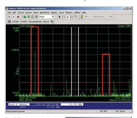
Figure 9. Alias checker results when the center frequency is originally tuned to an alias product. The checker shows no signal at the desired frequency (white solid/dashed box) and large zone boxes at the zones containing the desired signal.
