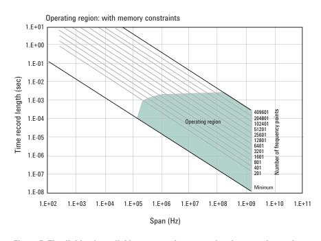
Figure 5. The digitizer's available memory also constrains the operating region
