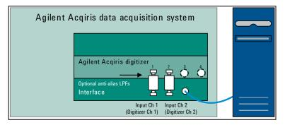
Figure 1a. Digitizers connected through CompactPCI to PCI interface
