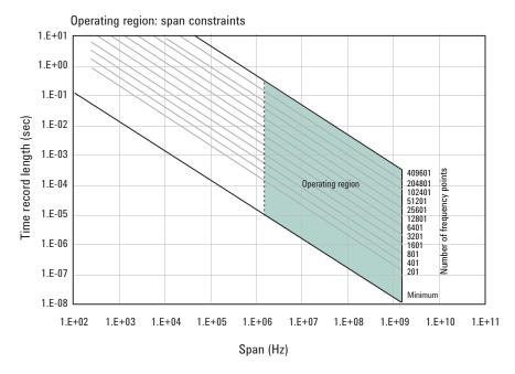
Figure 4. The allowable range of spans, which may differ by model, further bound the operating region of the digitizer
