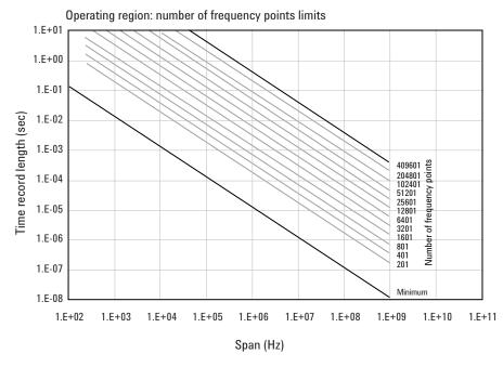
Figure 3. The user-settable parameter, frequency points, begins to determine the boundaries of the time record length and frequency span operating region
