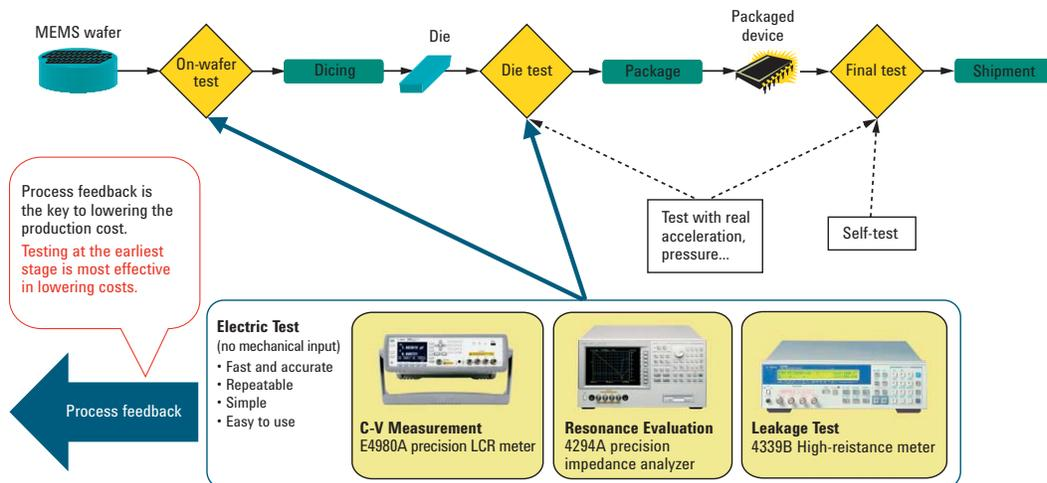
Figure 1. MEMS wafer characterization process
