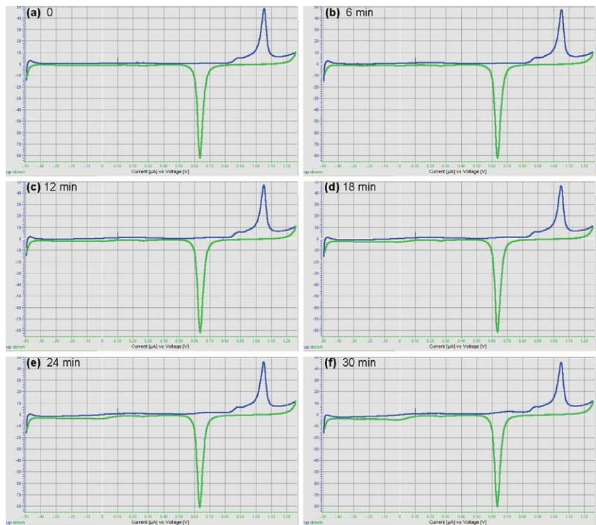
Figure 3. Continuous change in cyclic voltammograms after the nitrogen flow was completely stopped.
