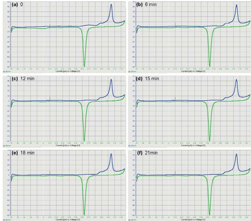
Figure 2. Continuous cyclic voltammograms in 21 minutes of purge from  $\sim 5\%$  oxygen concentration.
