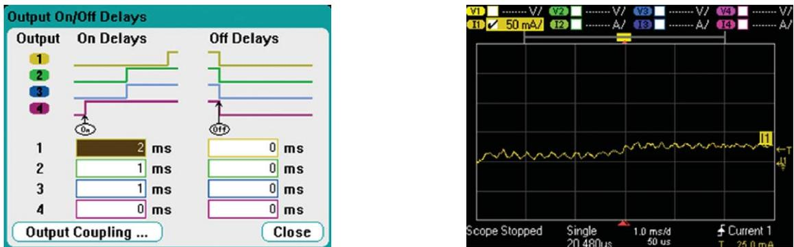
To achieve the ramp rate requirements for VCCINT and VCCO (see Figure 1), the slew rates for channels 1 and 2 were adjusted. Figure 4 shows the N6705A display for changing a channel's slew rate, which is expressed in volts per second (V/s).
