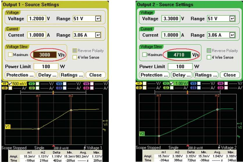
Figure 5: Power module voltages at turn-on
