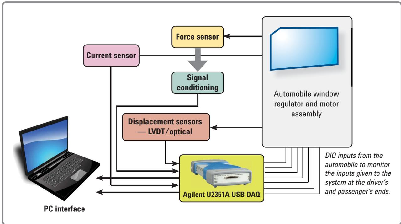
Figure 7. Application block diagram
