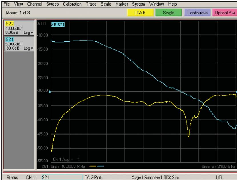
Figure 17. O/E responsivity and electrical return loss measurement
