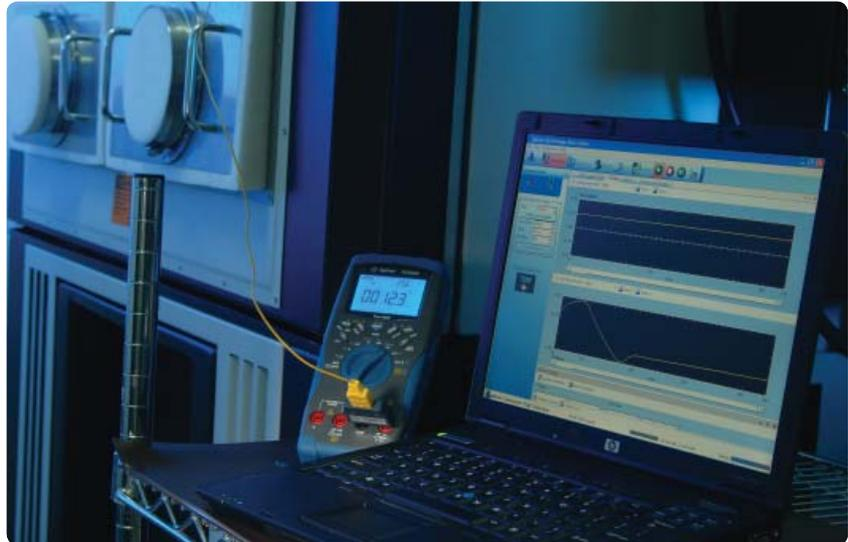
Figure 1. Performing data logging with the U1250A Series handheld DMM and the GUI datalogger software.
