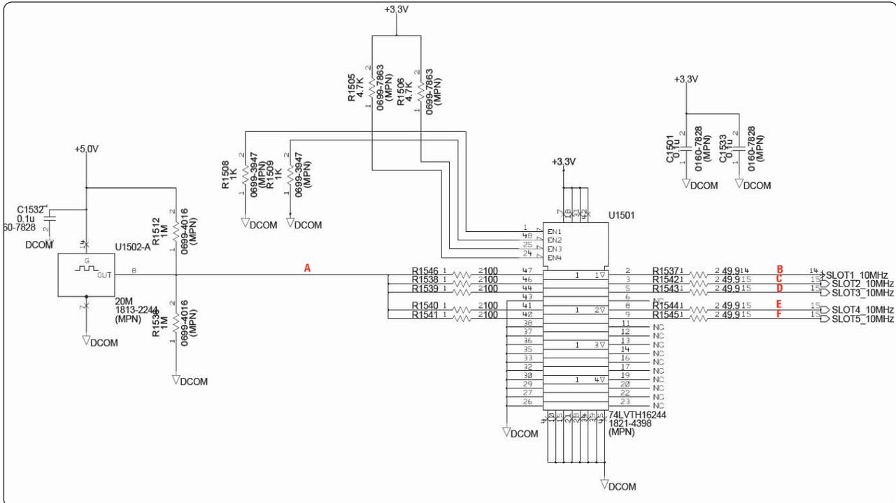
Figure 4. Reference clock schematic for carrier board
