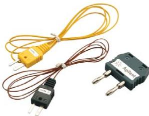
Thermocouple adapter is a cost effective solution to your temperature measuring needs. The Agilent U1180A thermocouple adapter and lead set includes a non-compensation transfer adapter, J-type and K-type thermocouple beads. The transfer adapter is used to convert the thermocouple's miniature connector to banana plugs (for adapting to the DMM's terminal). Both thermocouple J-type and K-type have effective temperature range of  $-20\text{ }^{\circ}\text{C}$  to  $200\text{ }^{\circ}\text{C}$ .
