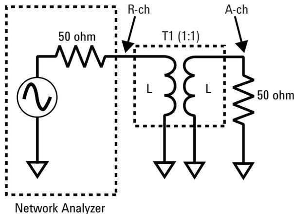
Figure 12. Evaluation method of the transformer's transmission characteristics
