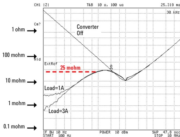
**Figure 25. Output impedance measurement example with shunt-thru method**
