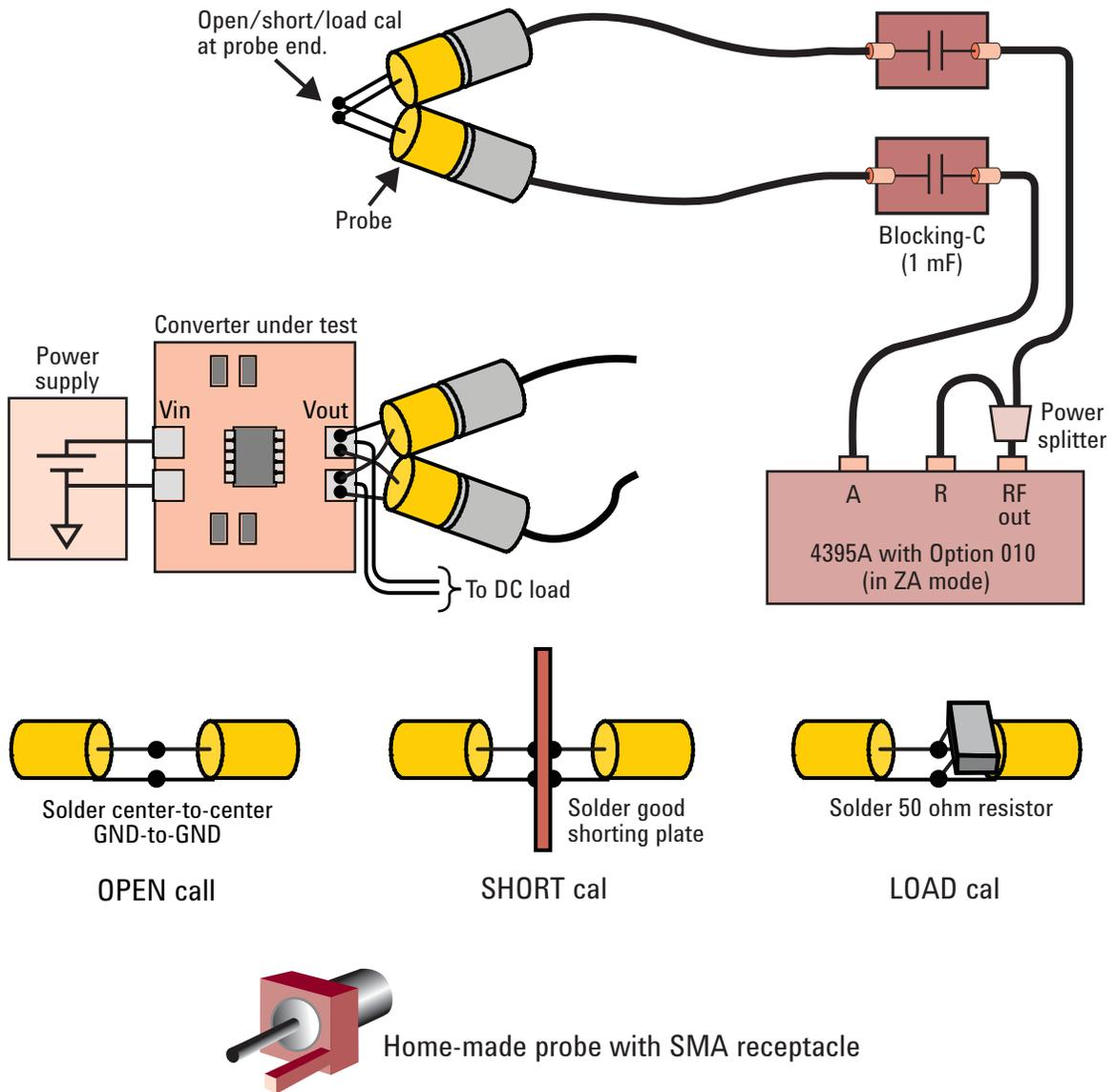
Figure 23. Example of probing method for shunt-thru method (1)
