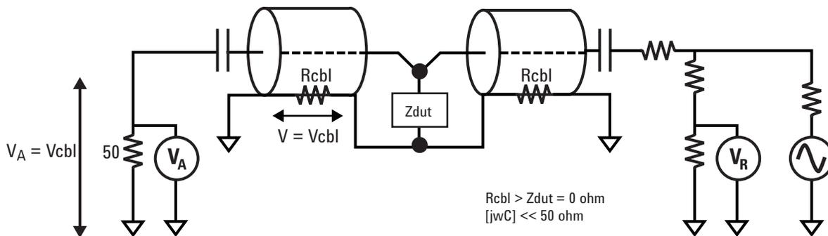
Figure 17. Error caused by cable braid impedance
