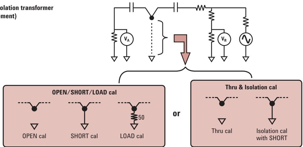
Figure 20. OPEN/SHORT/LOAD calibration, thru & isolation calibration
