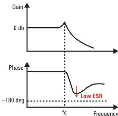
Figure 5. Gain-phase characteristics of output LC filter
