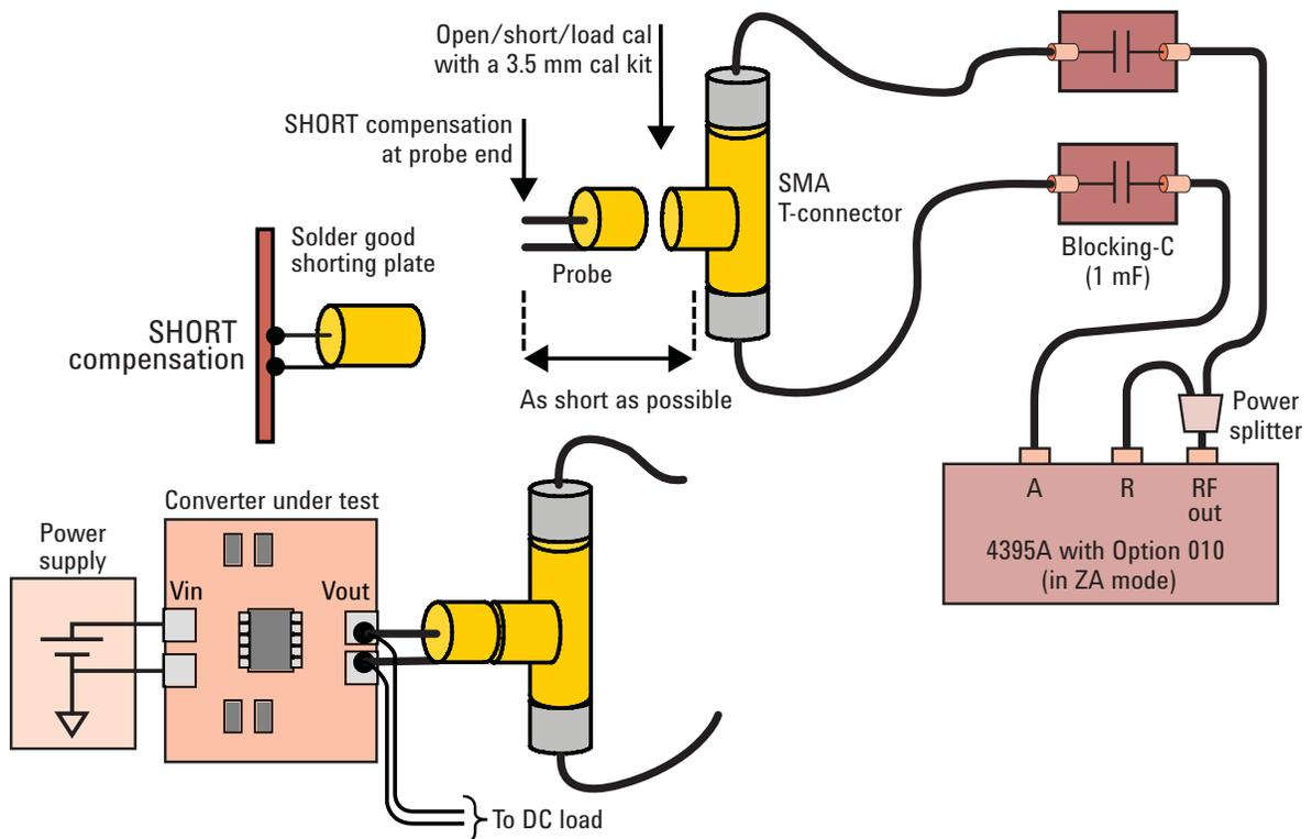
Figure 24. Example of probing method for shunt-thru method (2)
