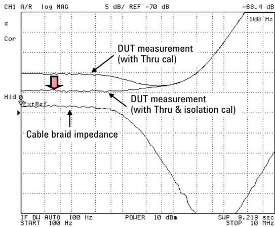
Figure 21. Calibration with SHORT device
