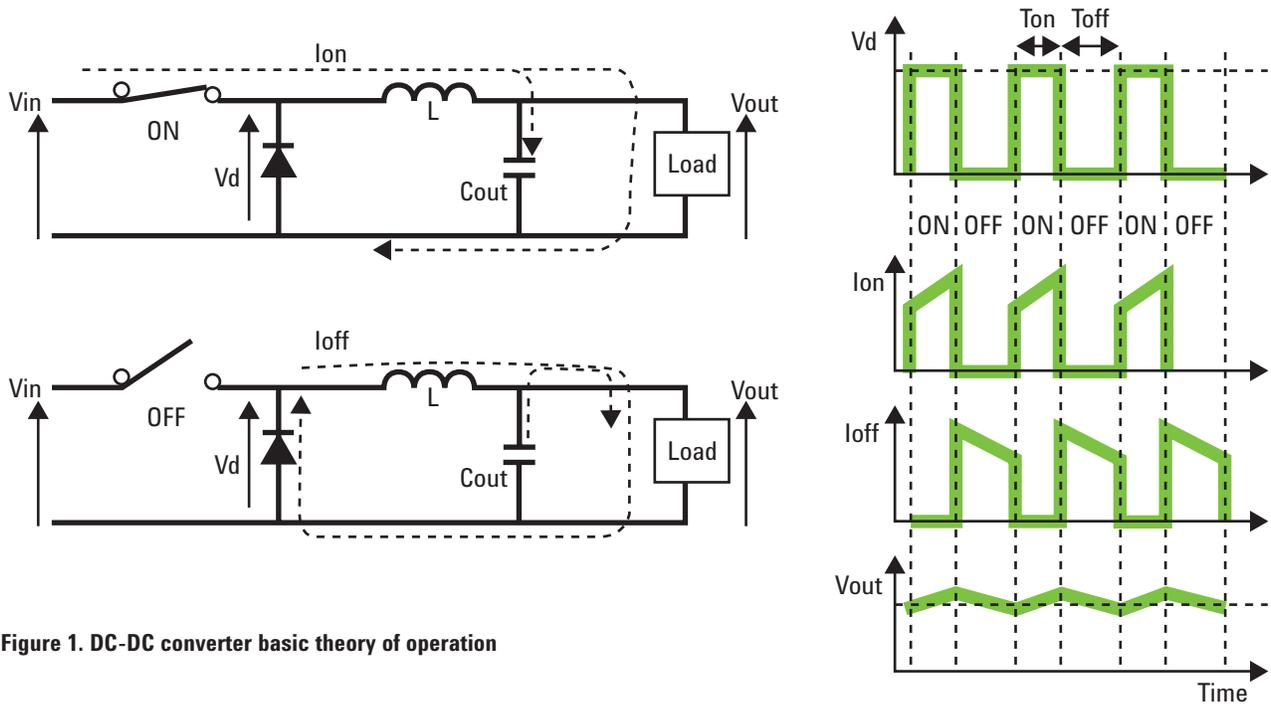
Figure 1. DC-DC converter basic theory of operation
