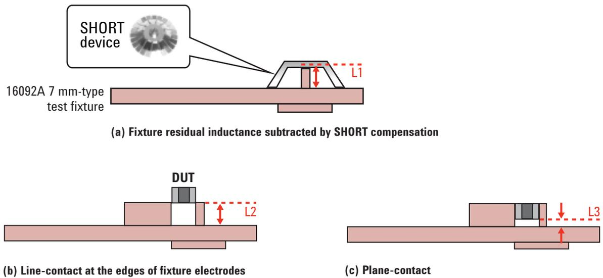
Figure 27. Tips for measuring low-ESR and low-ESL capacitors
