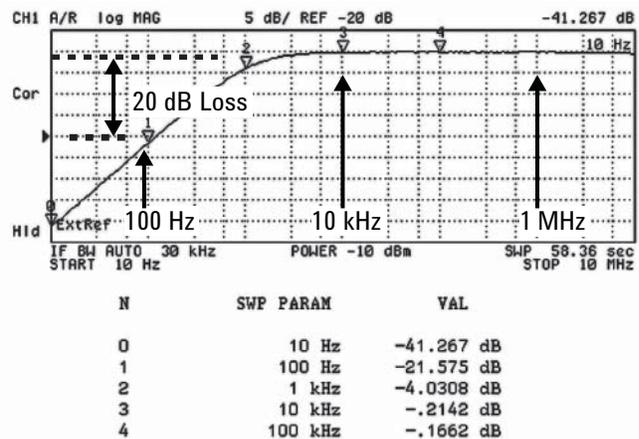
Figure 13. Transmission characteristic of pulse transformer (PN 9100-0855)
