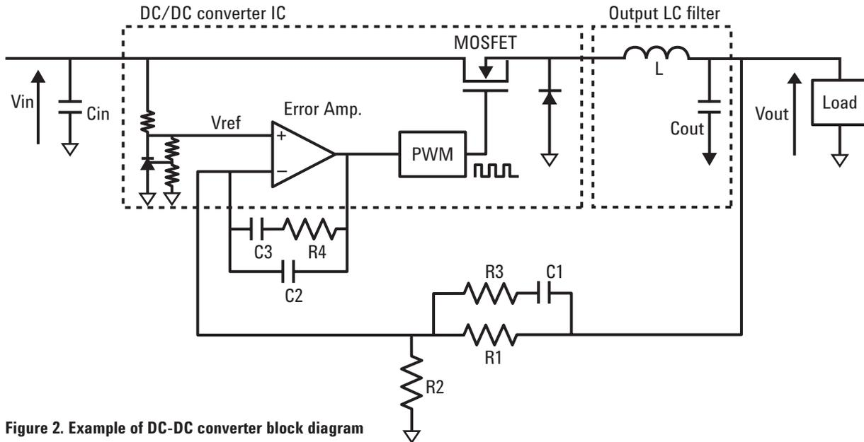
Figure 2. Example of DC-DC converter block diagram
