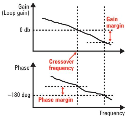
Figure 4. Gain-phase characteristics of  $GH$  (Bode plot)
