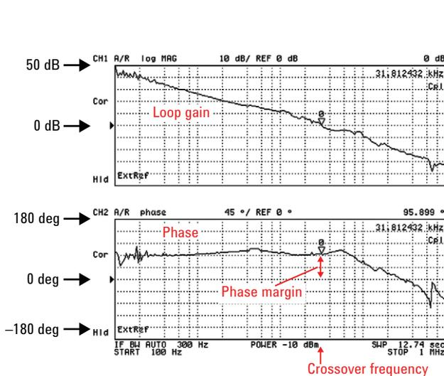
Figure 9. Loop gain measurement example of DC-DC converter
