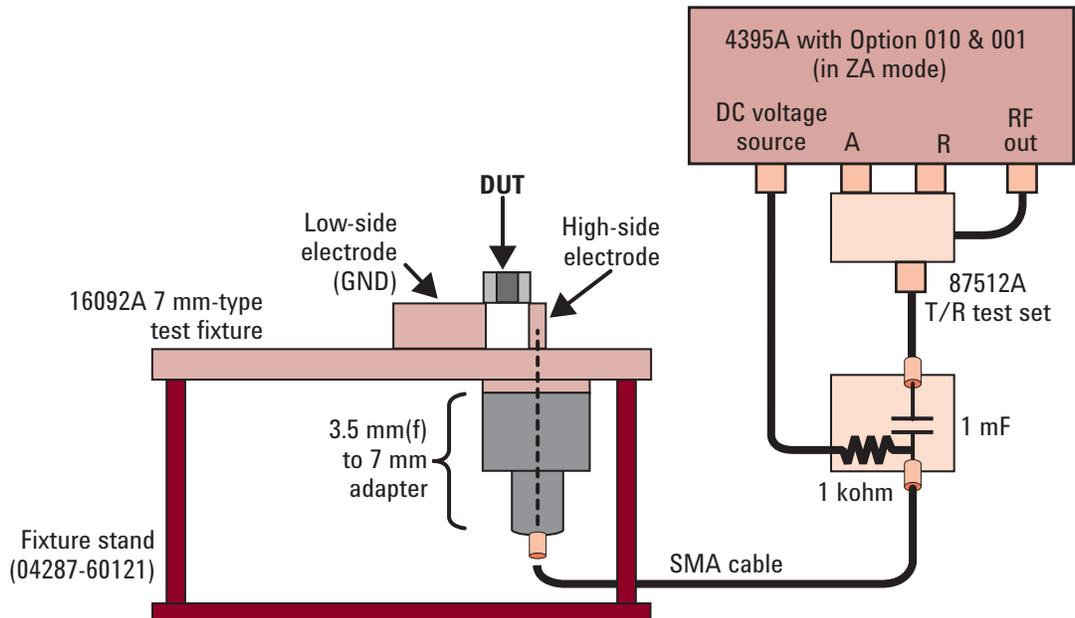
Figure 26. Configuration example for measuring passive component impedance
