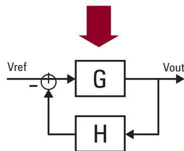
$$\frac{V_{out}}{V_{ref}} = \frac{G}{1+GH}$$
