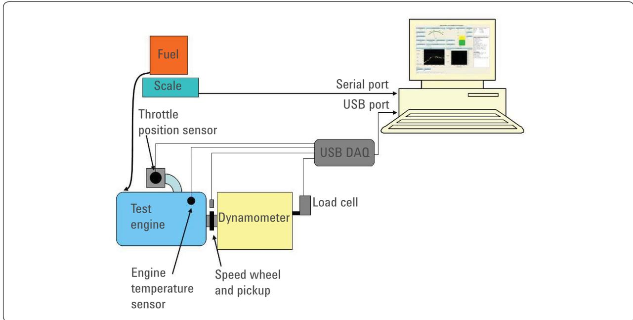
**Figure 1.** Schematic overview of test system
