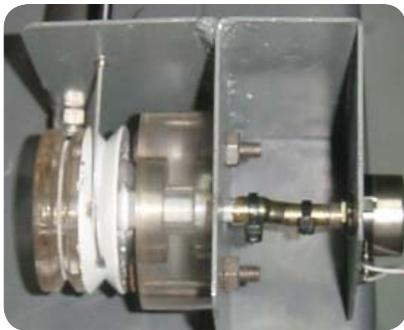
**Figure 5.** TPS pot (right) and throttle linkage (left)
