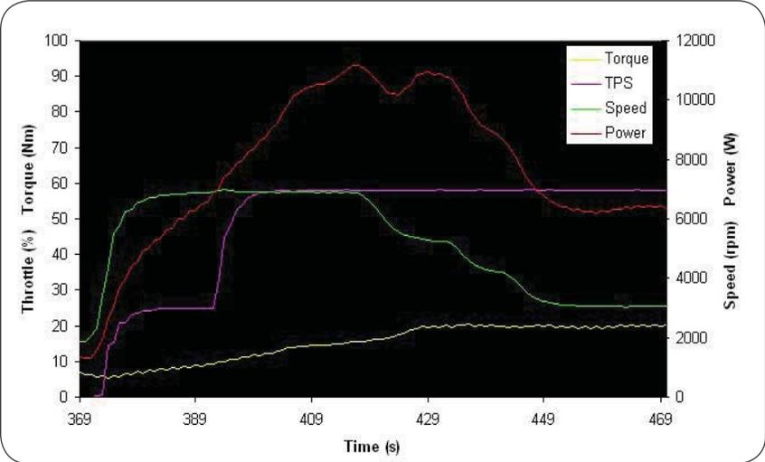
**Figure 10.** Post-processed data (from run shown above) with power calculated
