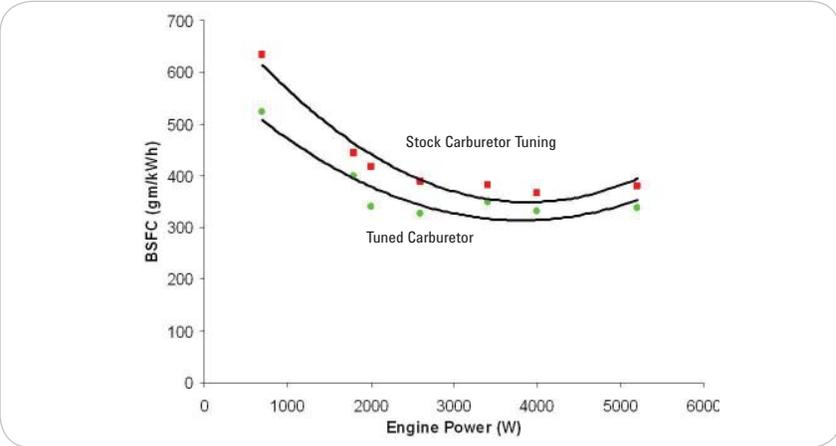
**Figure 12.** Brake-specific fuel consumption vs. engine power for stock and tuned carburetor
