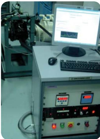
**Figure 6.** Controller in the foreground, engine and dynamometer behind
