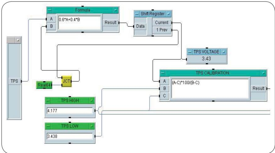
**Figure 8.** Exponential averaging and linear calibration of TPS value
