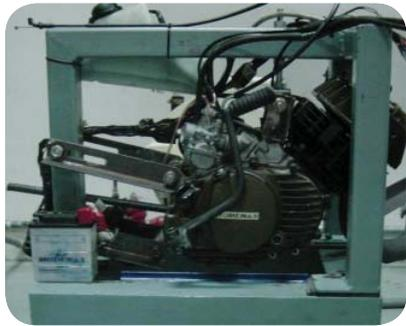
**Figure 2.** Motorcycle engine mounted for testing
