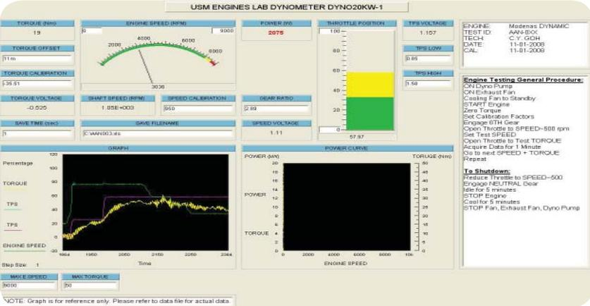
**Figure 9.** Computer screen with Agilent VEE front panel during engine testing
