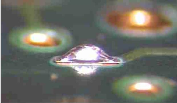
**Figure 3: A Bead Probe, approximately 5 mils by 20 mils, viewed at a 30 degree angle.**
