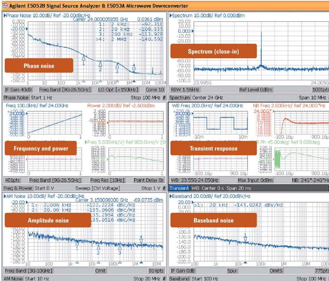
Figure 1. Six fundamental functions of the E5052B
