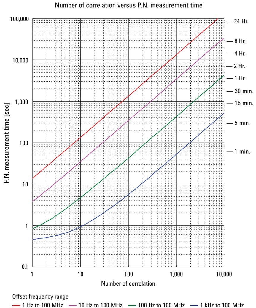
**Figure 4. Number of correlation versus PN measurement time**
