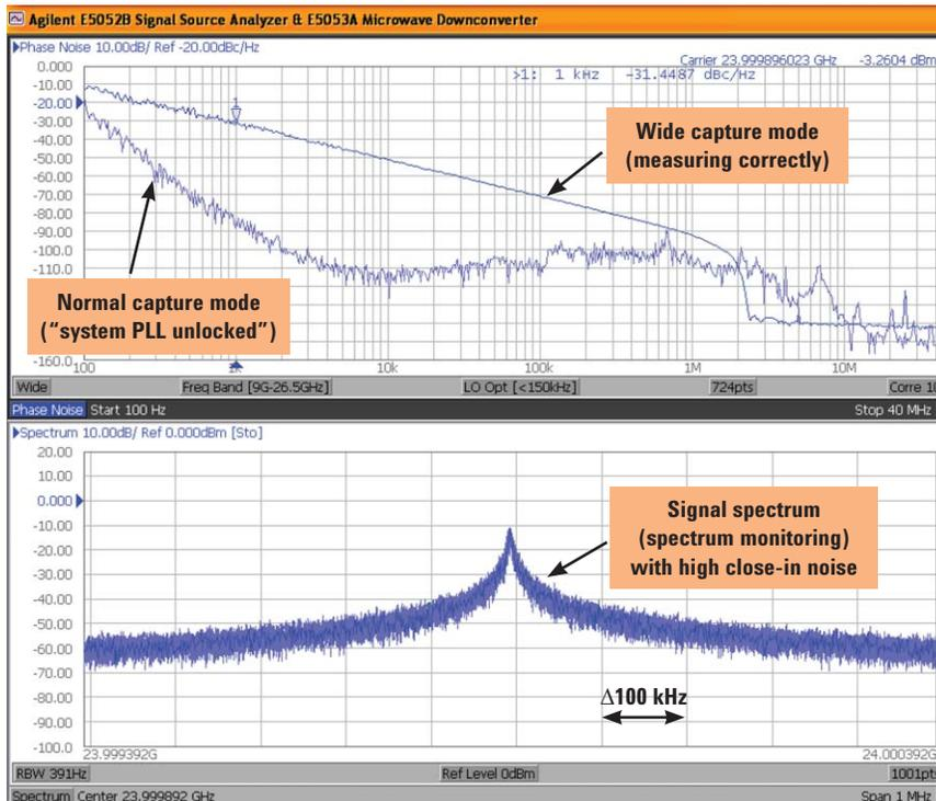
Figure 6. 24 GHz noisy signal source measurements
