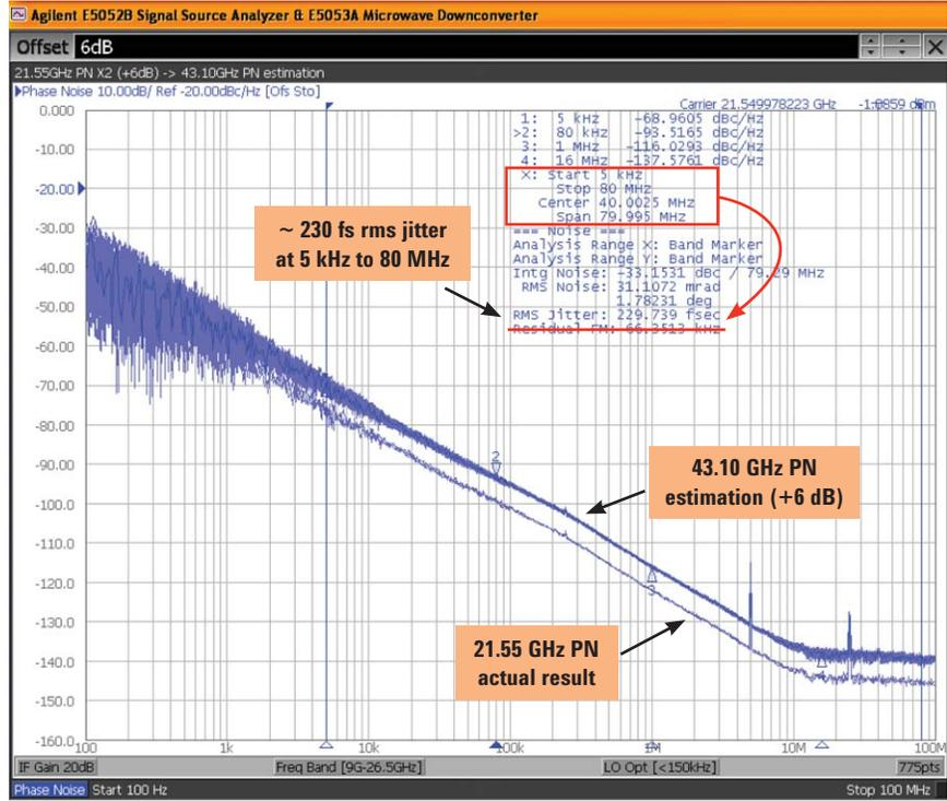
Figure 2. 21.55 GHz jitter measurement by the E5053A
