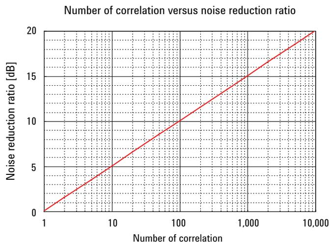
**Figure 5. Number of correlation versus noise reduction ratio**
