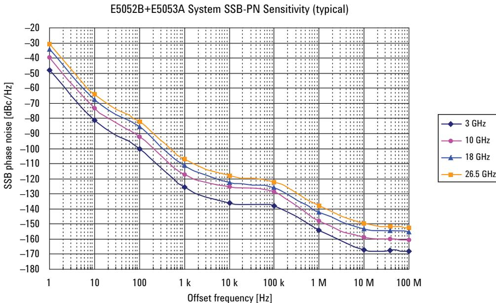
Figure 3. E5053A system phase noise floor
