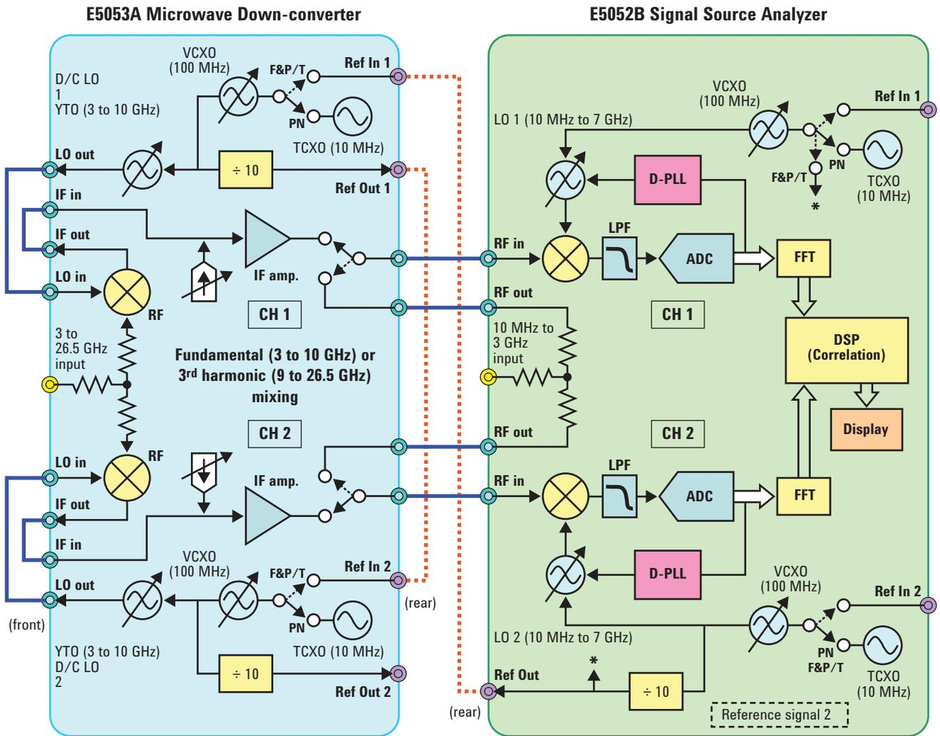
Figure 8. Internal reference signal connection diagram for E5053A + E5052B
