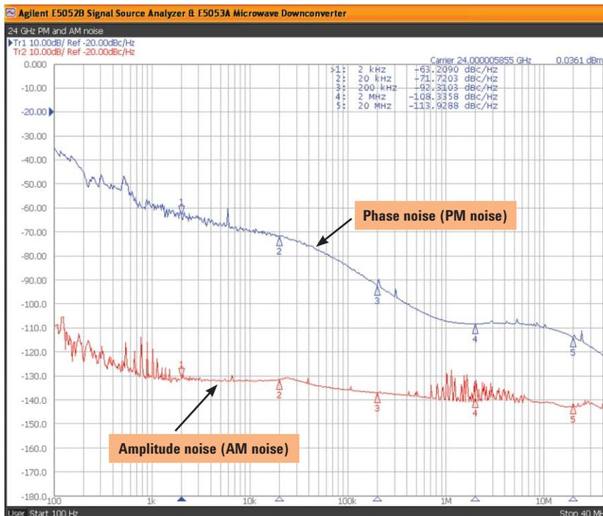
Figure 7. 24 GHz PM and AM noise
