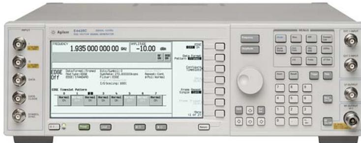
Figure 1. E4438C ESG vector signal generator
