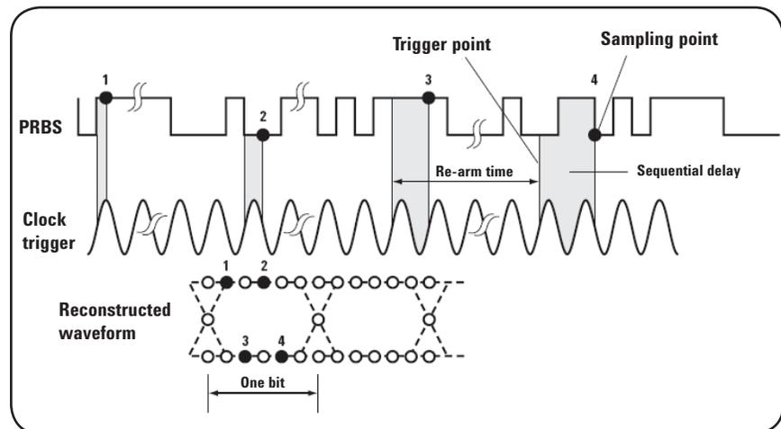
Figure 4 - Sampling Process for an Eye Diagram Waveform
