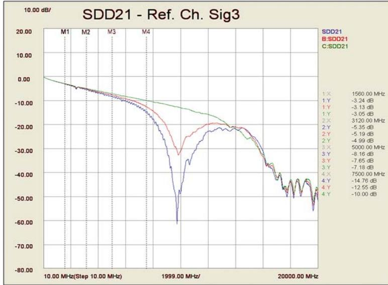
Figure 34. Reference Channel Insertion Loss with Trimmed SMA
