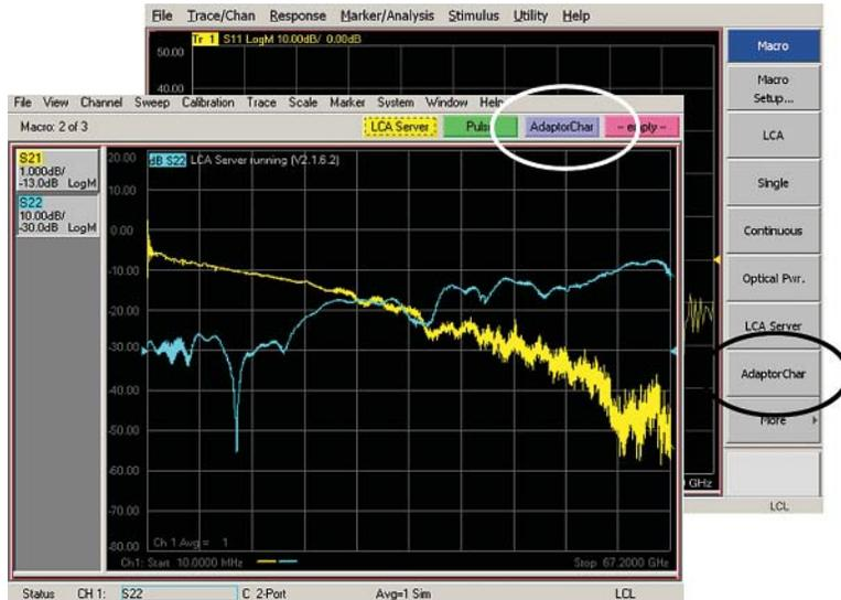
Figure 17. Adapter Characterization Macro Softkeys on PNA and PNA-X User interface
