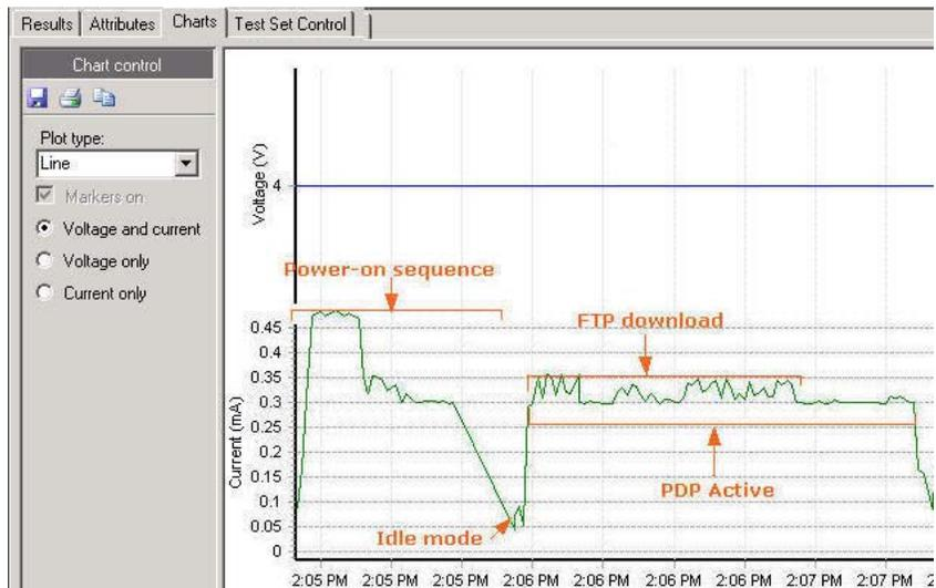
Figure 2: IFT generic battery current drain analysis view
