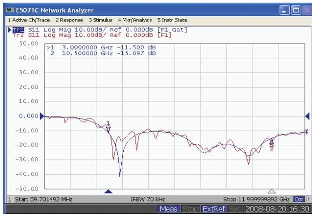
**Figure 4. Frequency domain with/without gating**
