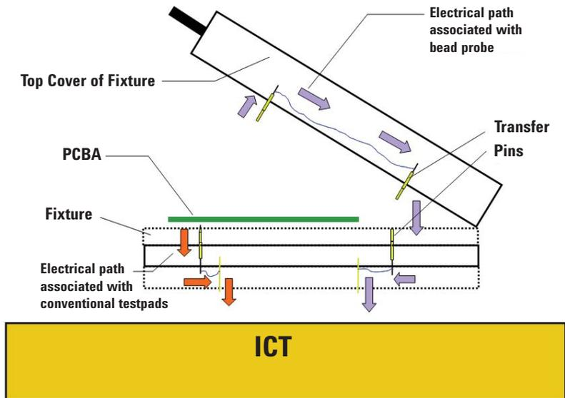
Figure 1 : Electrical path associated with the bead probe locations and conventional test pads
