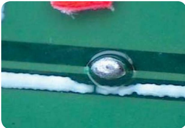
*Figure 2 : Bead probes before actuation at ICT*
