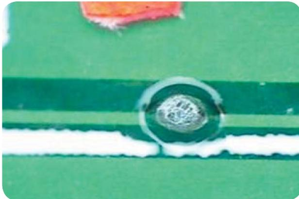
*Figure 3 : Bead probes after one actuation at ICT*
