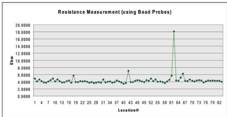
Figure 8 : Measurement of internal IC resistance using bead probes as test access
