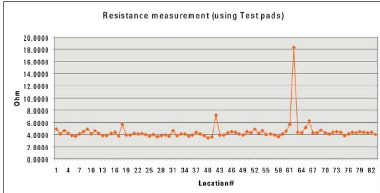
Figure 7 : Measurement of internal IC resistance using testpads as test access
