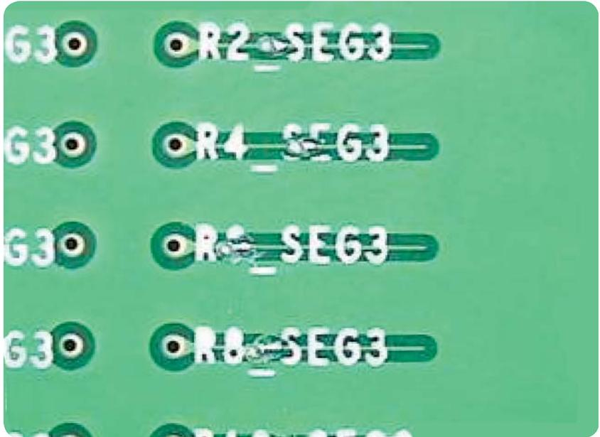
Figure 6 : A cluster of bead probes being pushed out of their position
