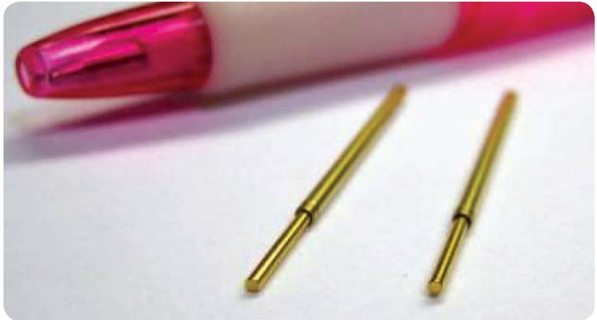
Figure 4 : Headless test probes were used on bead probe locations.
