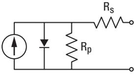
Figure 2: Solar cell circuit equivalent
