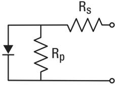
Figure 16: Solar cell equivalent circuit during dark testing
