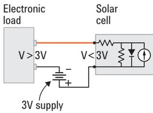
Figure 8: Electronic load configuration with 3-V boost supply
