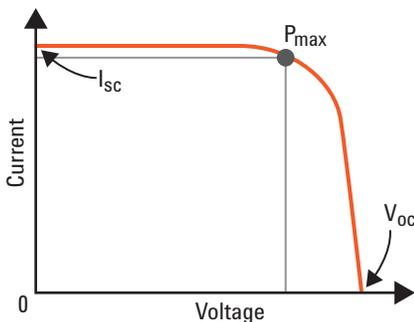
Figure 1: Solar cell I-V curve
