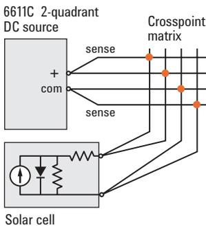
Figure 4a: Solar cell electrical characterization test setup configured to capture the I-V curve of a solar cell
