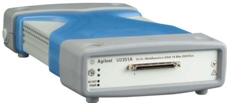
Figure 1. The Agilent U2351A DAQ
