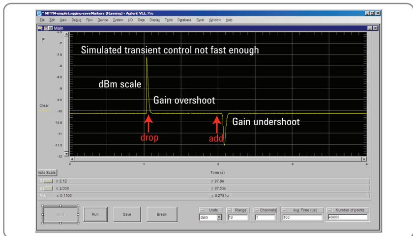
Figure 5. EDFA transients: 2-wavelength method.
